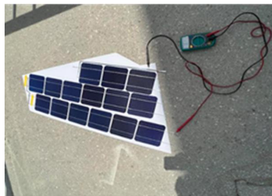
Fig. 10 Testing of PV cells output from one wing which are connected one in series
