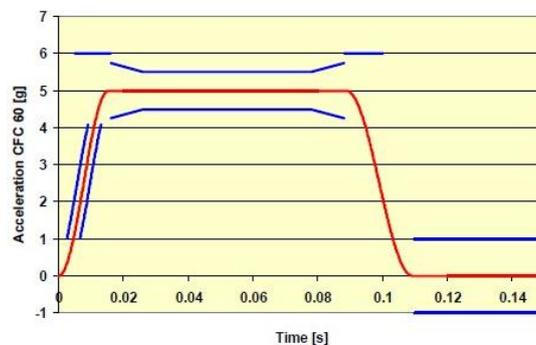
Fig. 8 Low severity pulse of the euro NCAP whiplash test protocol
