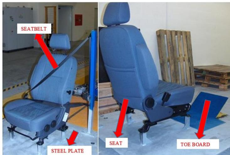
Fig. 4 Test sample elements
