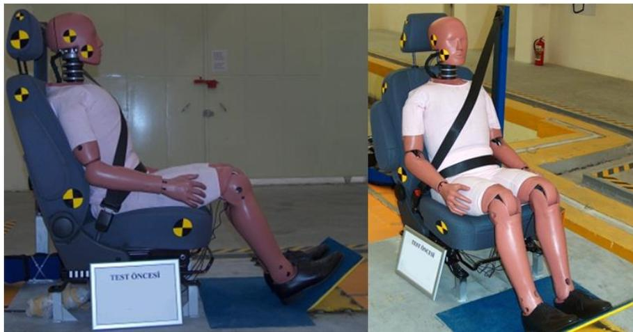
Fig. 7 Positioned dummy in the seat
