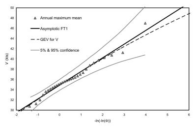
Fig. 2 Gumbel plot for annual maximum hourly mean wind speeds from observed annual maxima at Boscombe Down
