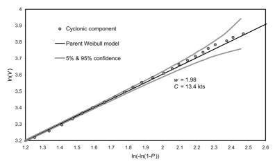
Fig. 1 Upper tail of Weibull plot of cyclonic component of parent mean wind speed (>25 kts) with bootstrap confidence limits
