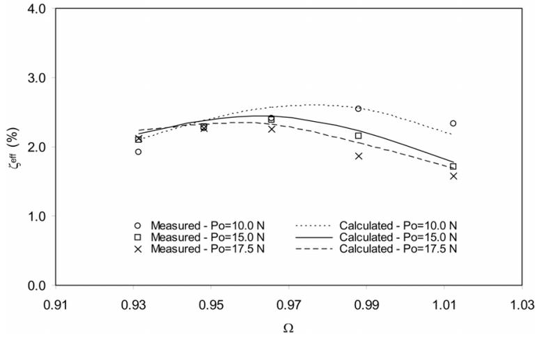
Fig. 11 Comparison of effective damping values from equivalent TMD model and experiments
