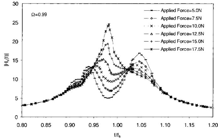
Fig. 3 Mechanical admittance function of structure-TLD system with varying excitation amplitudes
