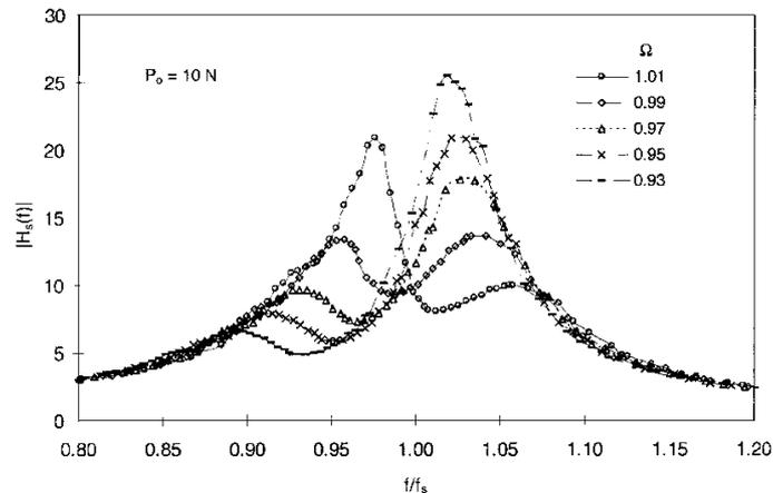
Fig. 4 Mechanical admittance function of structure-TLD system with varying tuning ratio values
