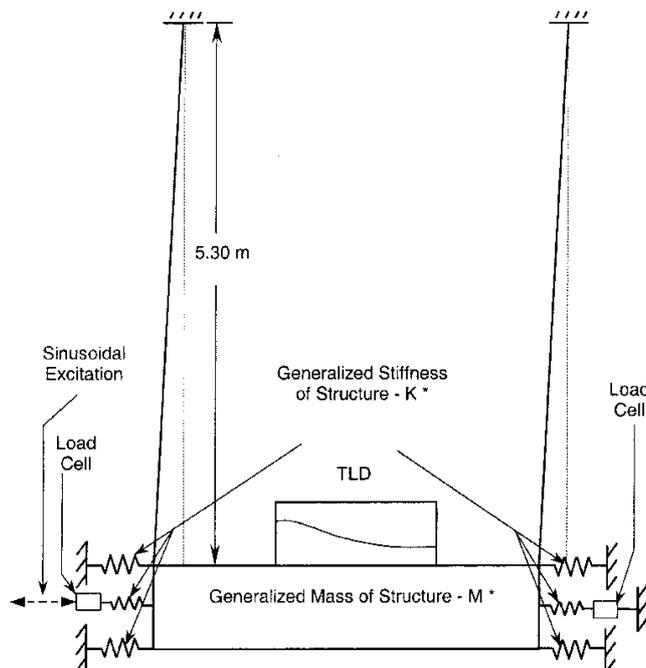
Fig. 1 Schematic of two degree of freedom structure-TLD system
