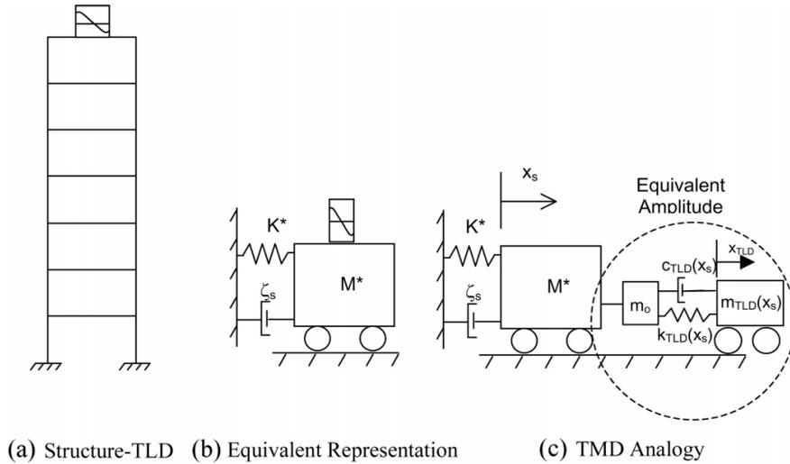
Fig. 7 (a) Structures-TLD, (b) equivalent representation, (c) TMD analogy
