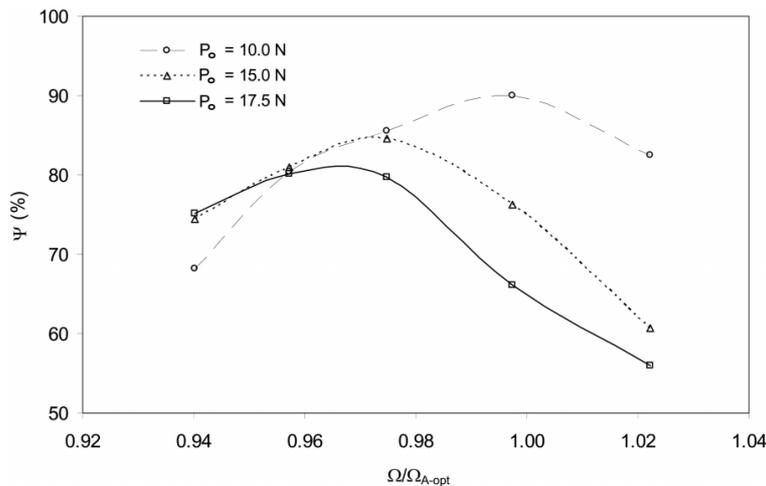
Fig. 5 Influence of tuning ratio on the efficiency of a TLD for different excitation amplitudes
