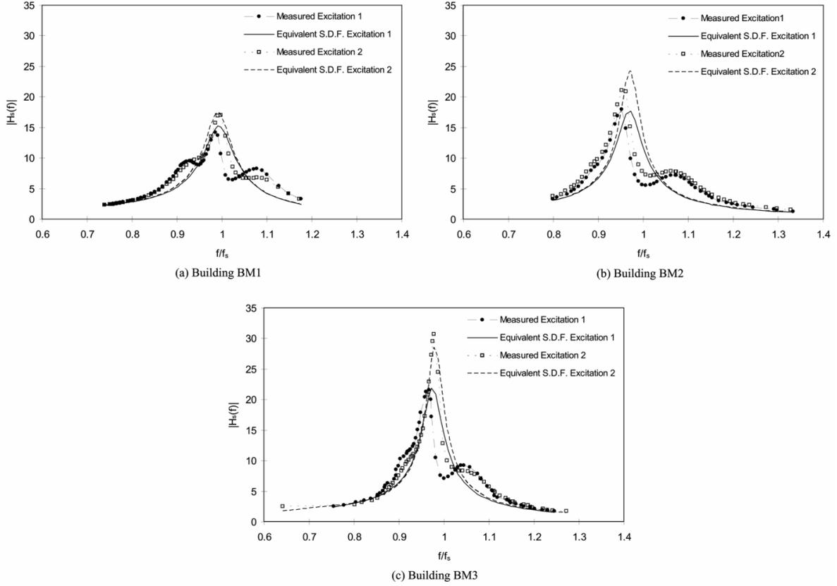
Fig. 2 Mechanical admittance functions for 3 model buildings for 2 different excitation amplitudes
