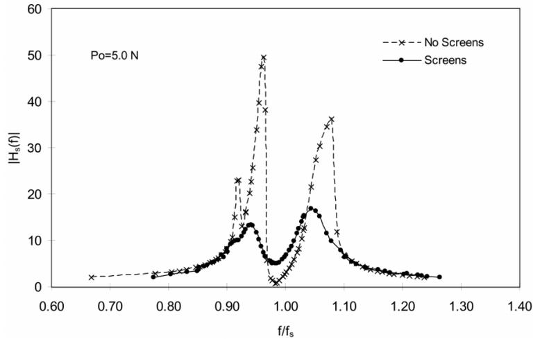
Fig. 6 Influence of damping screens on structural response
