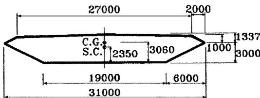
Fig. 1 Cross section of the Great Belt East Bridge suspension span. All dimensions are in mm
