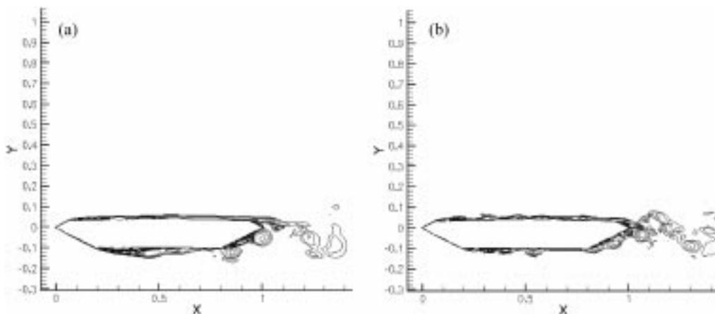
Fig. 4 Vorticity contour diagram using (a) LES model (b) no LES model
