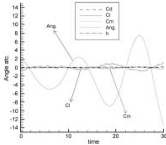
Fig. 6 Bridge response for reduced velocity  $u^*$  of 1.4 (flutter condition)
