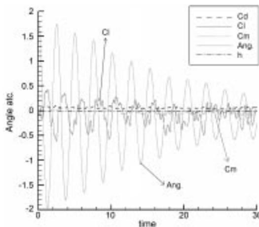
Fig. 5 Bridge response for reduced velocity  $u^*$  of 0.4 (no flutter condition)
