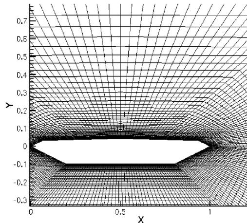
Fig. 3 Finite element grid for GBEB suspension span
