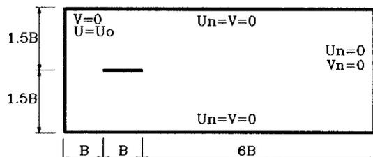
Fig. 2. Solution region and boundary conditions
