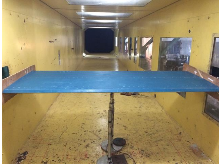
Fig. 11 Section model in wind tunnel
