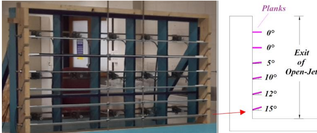
Fig. 6 Arrangement of passive planks used for adjusting wind velocity profile; (left): front view; (right): lateral elevation
