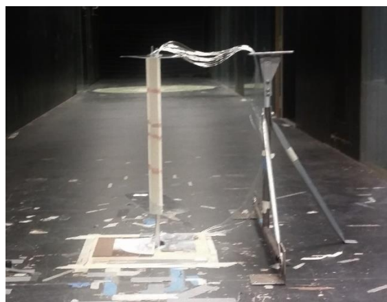
Fig. 9 Airfoil model in wind tunnel as mounted on the 3DOF system (underneath the test section) with a stand for supporting the pressure tubes (upstream view)
