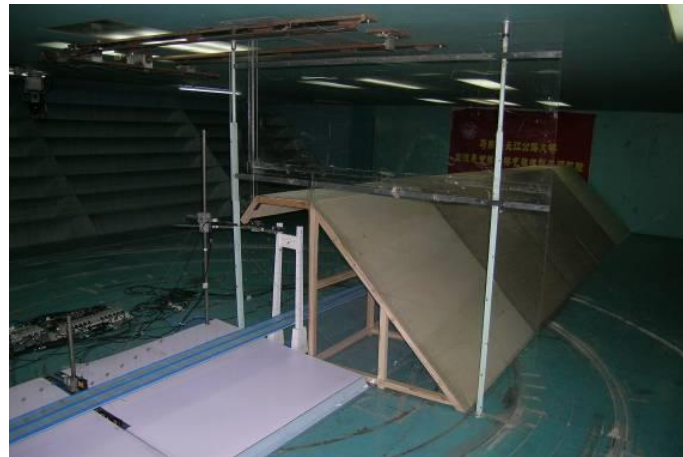
Fig. 10 Wind deflector, wind separating board and bridge model in wind tunnel
