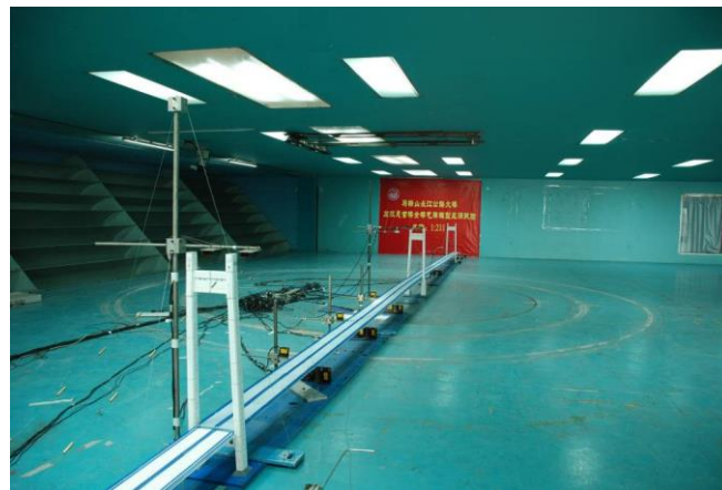
Fig. 3 Full bridge aeroelastic model in TJ-3 wind tunnel
