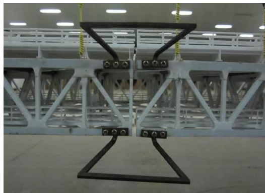
Fig. 10 Section girder model
