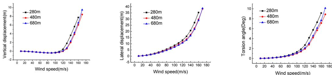
Fig. 6 Effect of the earth-anchored girder length on the girder displacement at midspan
