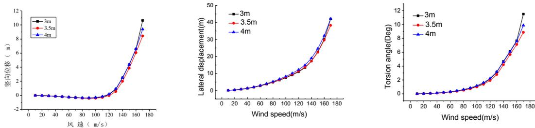
Fig. 9 Effect of the girder depth on the girder displacement at midspan
