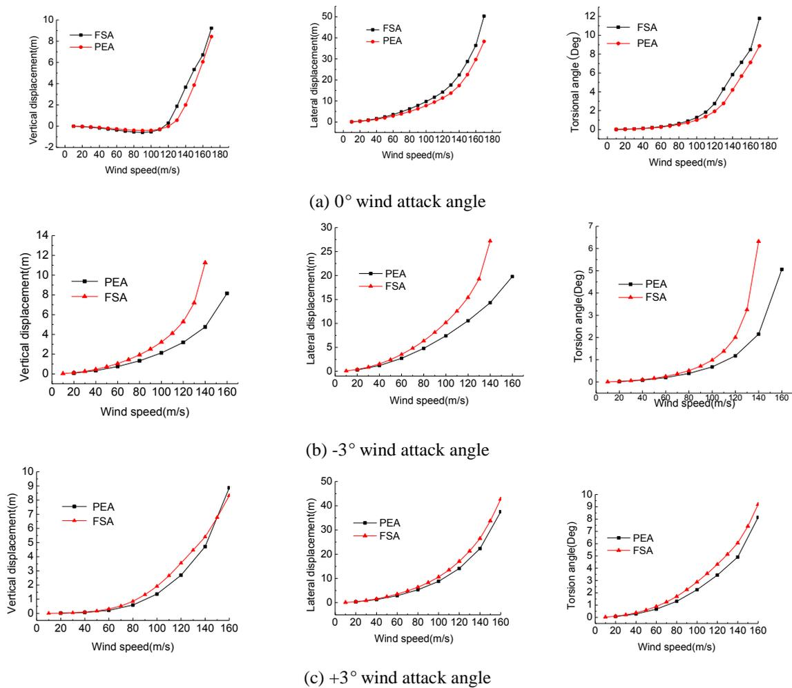
Fig. 4 Comparison of the girder displacement at midspan between the fully self-anchored and partially earth-anchored cable-stayed bridges under different wind attack angles
