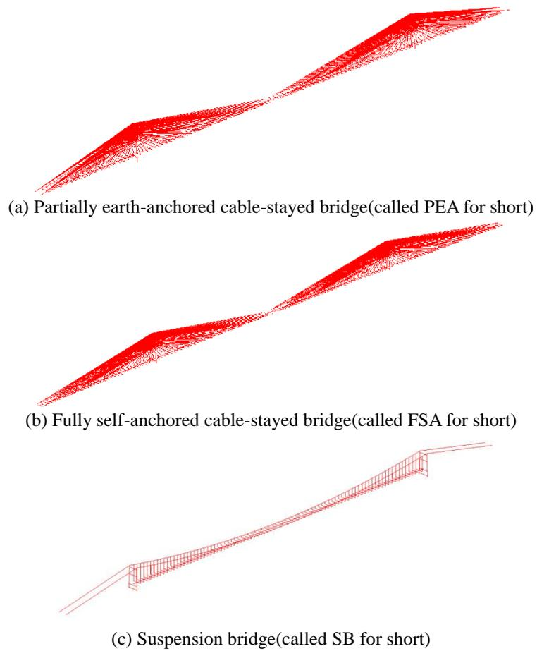
Fig. 3 Three-dimensional finite element models of the example bridges
