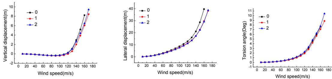
Fig. 7 Effect of the auxiliary piers on the girder displacement at midspan
