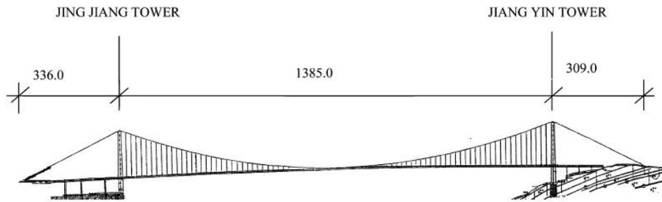
Fig. 2 General layout of the Jiangyin Bridge over the Yangtze River (unit: m)
