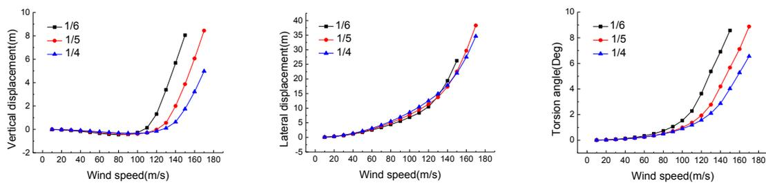
Fig. 10 Effect of the tower height-to-span ratio on the girder displacement at midspan
