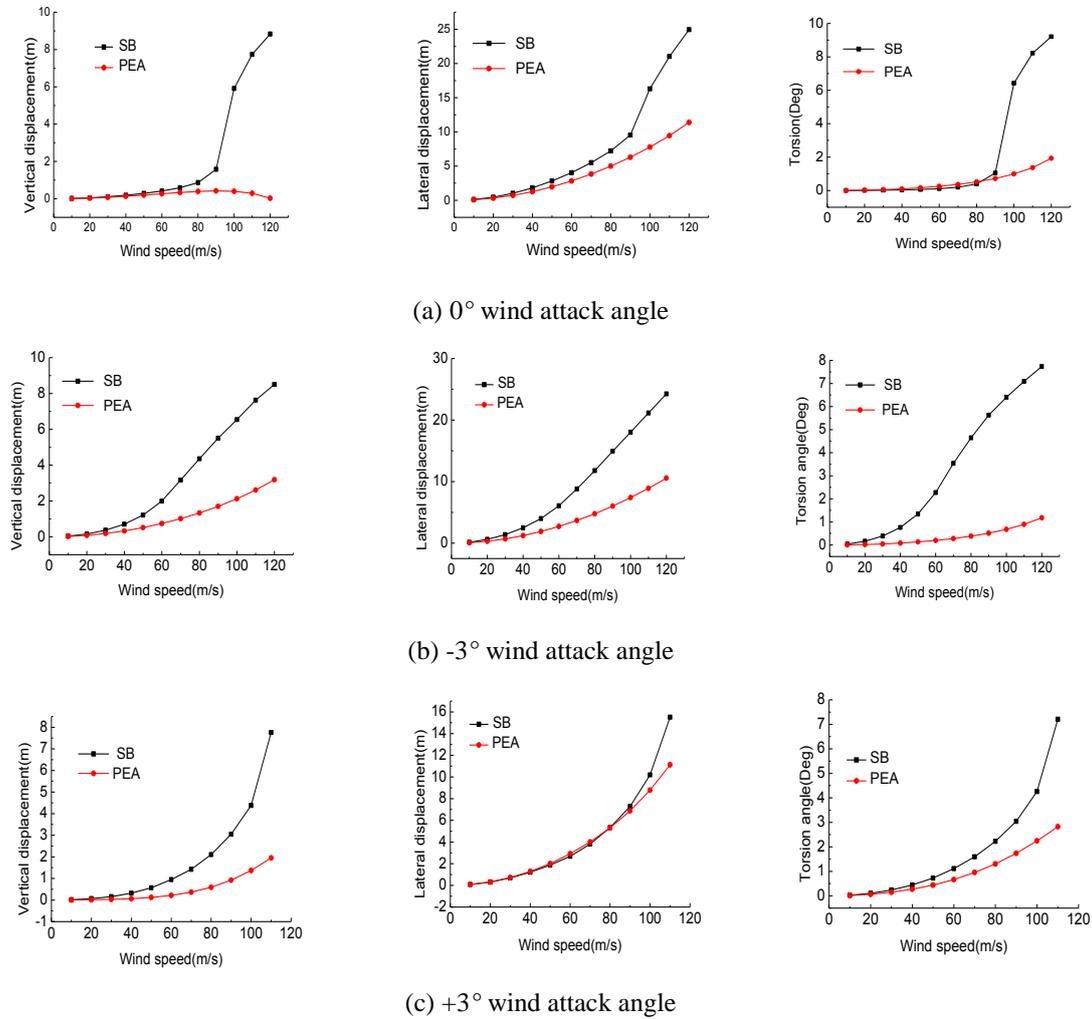
Fig. 5 Comparison of the girder displacement at midpoint between the partially earth-anchored cable-stayed bridge and suspension bridge under different wind attack angles
