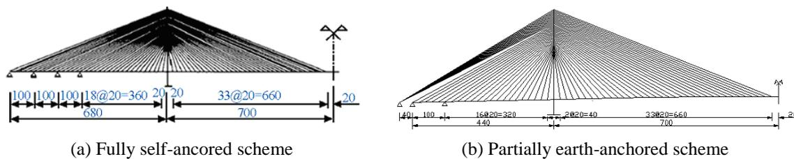
Fig. 1 General layout of super long-span cable-stayed bridge with 1400 m main span(half bridge)(unit: m)
