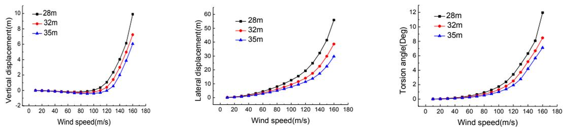
Fig. 8 Effect of the girder width on the girder displacement at midspan
