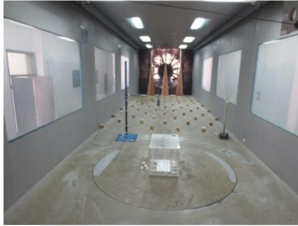
Fig. 2 Building model in the wind tunnel testing
