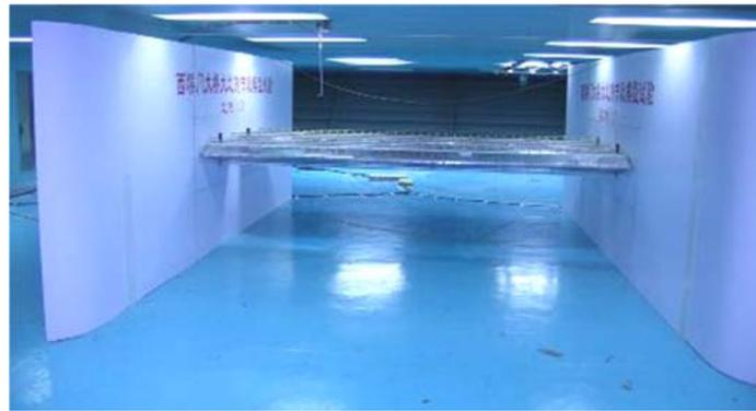
Fig. 7 The 1:20 girder sectional model
