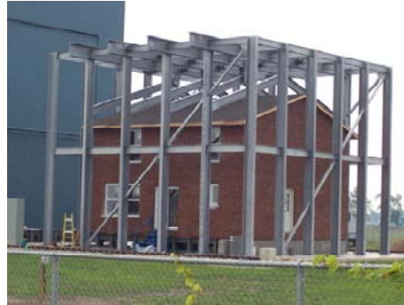
Fig. 1 Full-scale experimental set-up with steel reaction frame ( http://www.eng.uwo.ca/irlbh/ )
