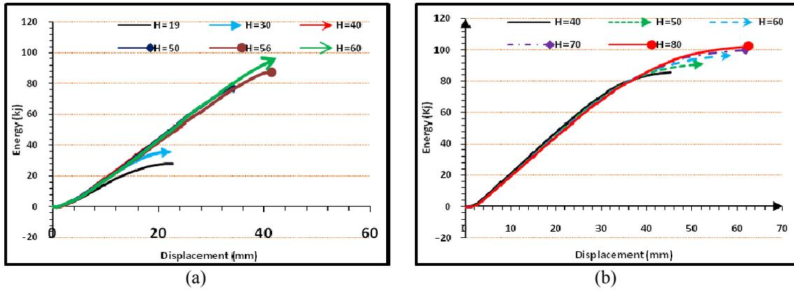
Fig. 10 Energy- displacement curves of (a) sinusoidal (b) trapezoidal corrugated plates with different corrugation depth
