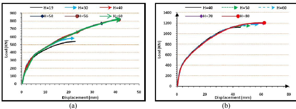
Fig. 9 Load- displacement curves of (a) sinusoidal (b) trapezoidal corrugated plates with different corrugation depth
