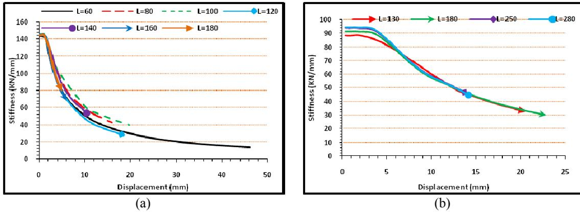
Fig. 14 Performance of stiffness curves of (a) sinusoidal (b) trapezoidal corrugated plates with different corrugation length
