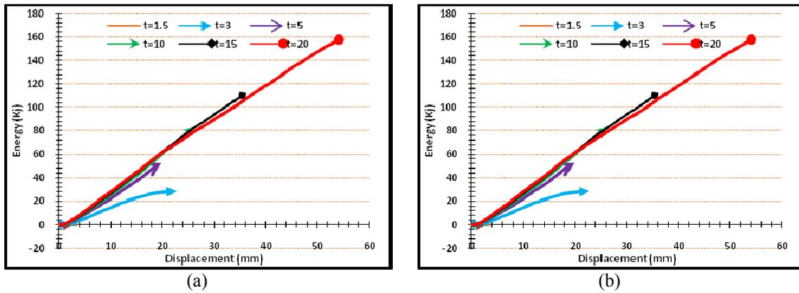
Fig. 7 Energy- displacement curves of (a) sinusoidal (b) trapezoidal corrugated plates with different thickness
