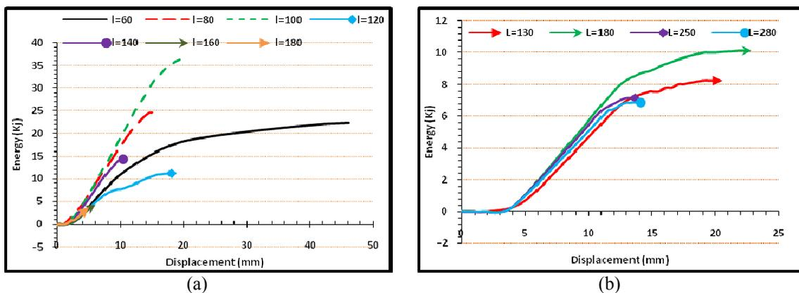
Fig. 13 Energy- displacement curves of (a) sinusoidal (b) trapezoidal corrugated plates with different corrugation length
