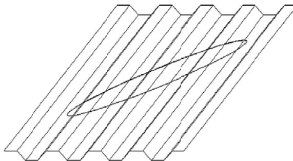
Fig. 4 Global buckling on trapezoidal corrugated plate
