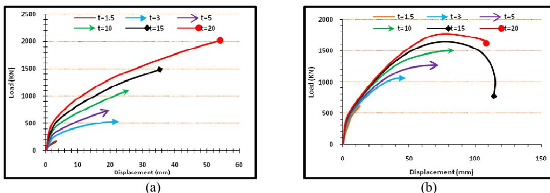
Fig. 6 Load- displacement curves of (a) sinusoidal (b) trapezoidal corrugated plates with different thickness
