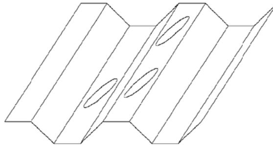
Fig. 3 The local buckling form in corrugates of plate
