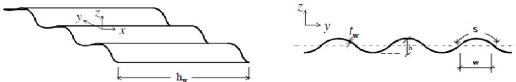
Fig. 2 Geometric properties of sinusoidal corrugated plate
