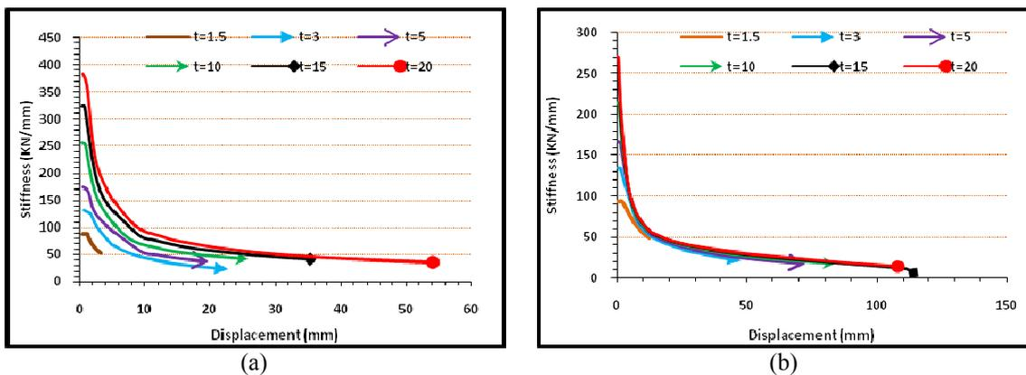
Fig. 8 performance of stiffness in (a) sinusoidal (b) trapezoidal corrugated plates with different thickness
