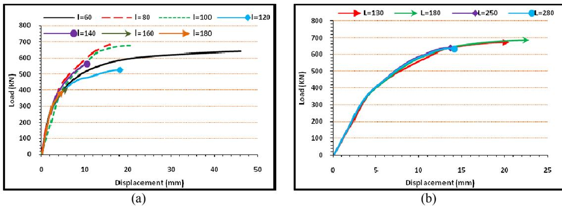
Fig. 12 Load- displacement curves of (a) sinusoidal (b) trapezoidal corrugated plates with different corrugation length
