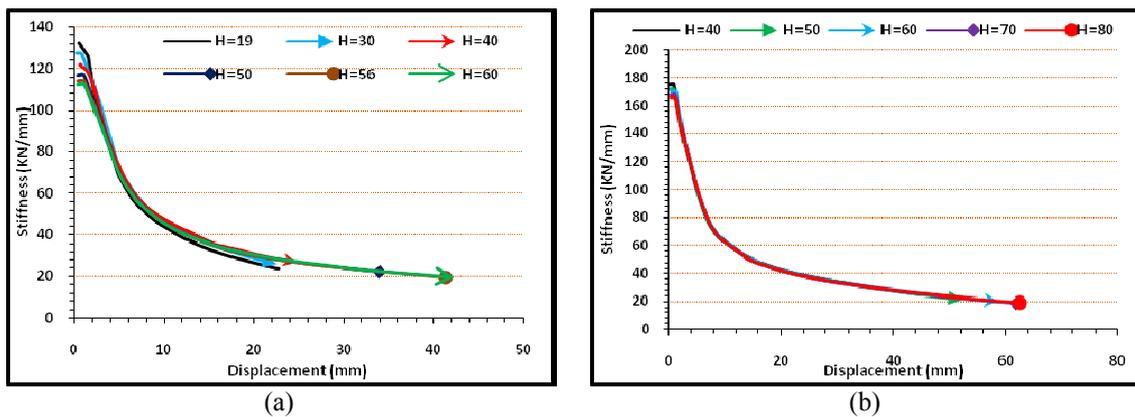
Fig. 11 Performance of stiffness curves (a) sinusoidal (b) trapezoidal corrugated plates with different corrugation depth
