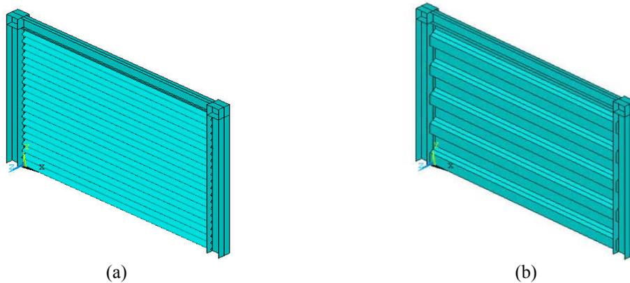
Fig. 5 the schematic corrugated steel shear wall with a) sinusoidal and b) trapezoidal waves
