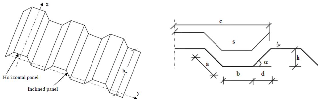
Fig. 1 Geometric properties of trapezoidal corrugated plate
