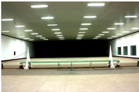
Fig. 9 View of full bridge model at XNJD-3 wind tunnel
