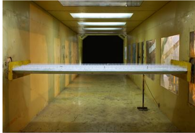
Fig. 3 View of section model in XNJD-1 wind tunnel
