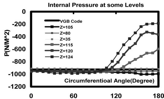
Fig. 3 Circumferential distribution of internal computed pressure at some levels of NDCT
