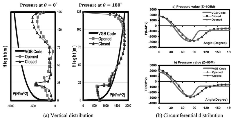
Fig. 1 Computed pressure of full scale NDCT for both closed and opened top conditions
