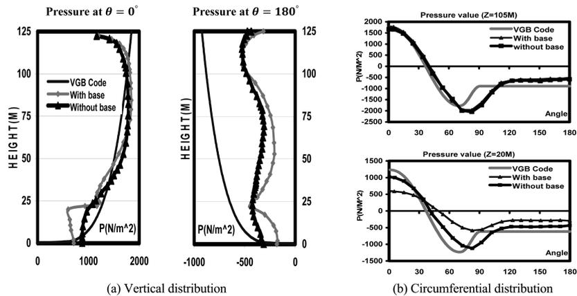
Fig. 5 Computed pressure of full scale NDCT for both with and without base structure
