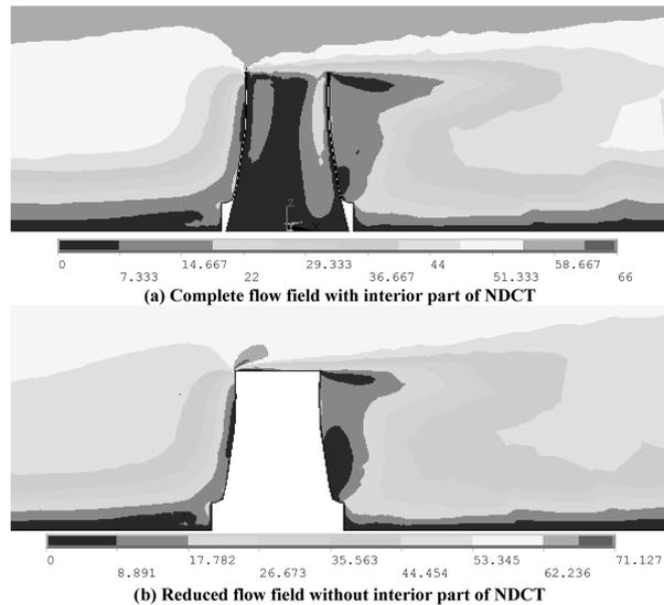
Fig. 2 Two dimensional color-coded computed velocity contours on a full NDCT external surface
