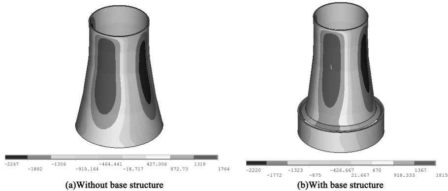
Fig. 4 Three dimensional color coded map of pressure on external surface of NDCT
