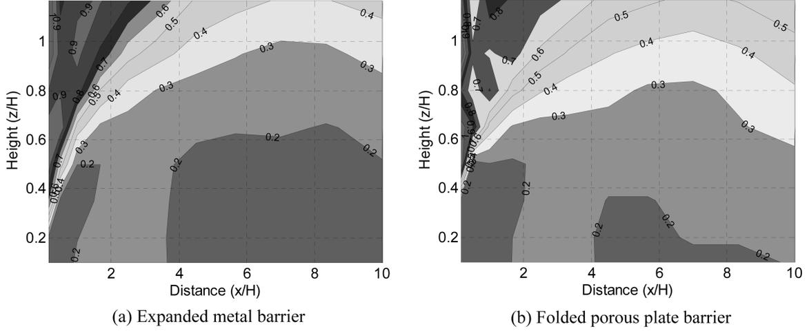
Fig. 12 Normalized wind velocities ( $V/V_\infty$ ) behind the wind barrier installed at embankment
