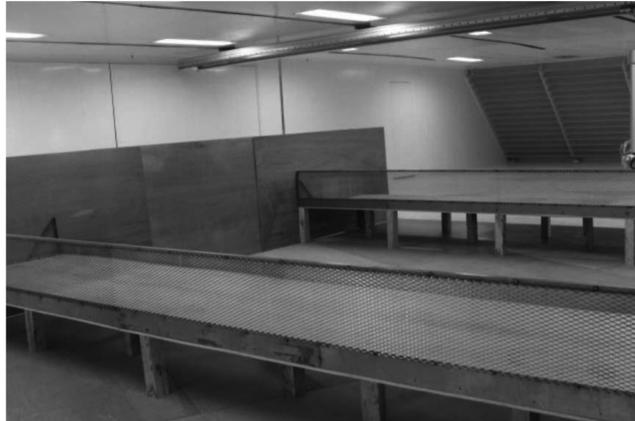
Fig. 14 Wind tunnel test of wind barriers at parallel bridges
