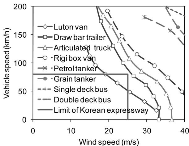
Fig. 2 Crosswind speed required to cause vehicle overtuning (Carr *et al.* 1993)
