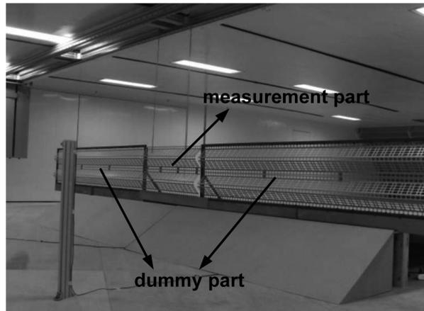
Fig. 13 Measurement of wind force acting on wind barrier
