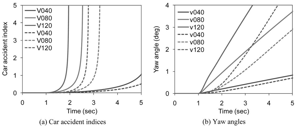
Fig. 7 Car accident indices and yaw angles of a sedan under wind action. Solid line: wind suddenly increased from 0 to 30 m/s, dotted line: wind linearly increased from 0 to 30 m/s for 3 seconds
