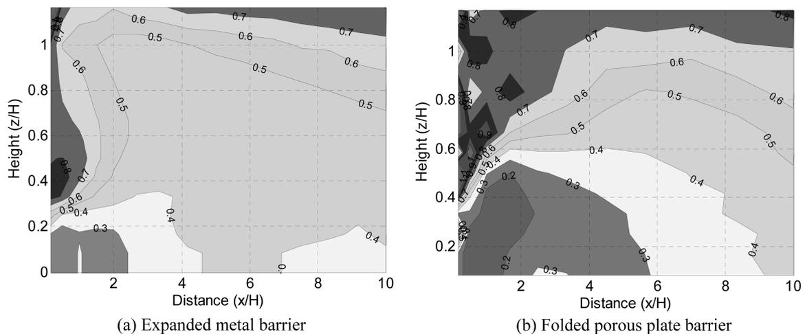
Fig. 11 Normalized wind velocities ( $V/V_\infty$ ) behind the wind barrier installed at elevated bridge
