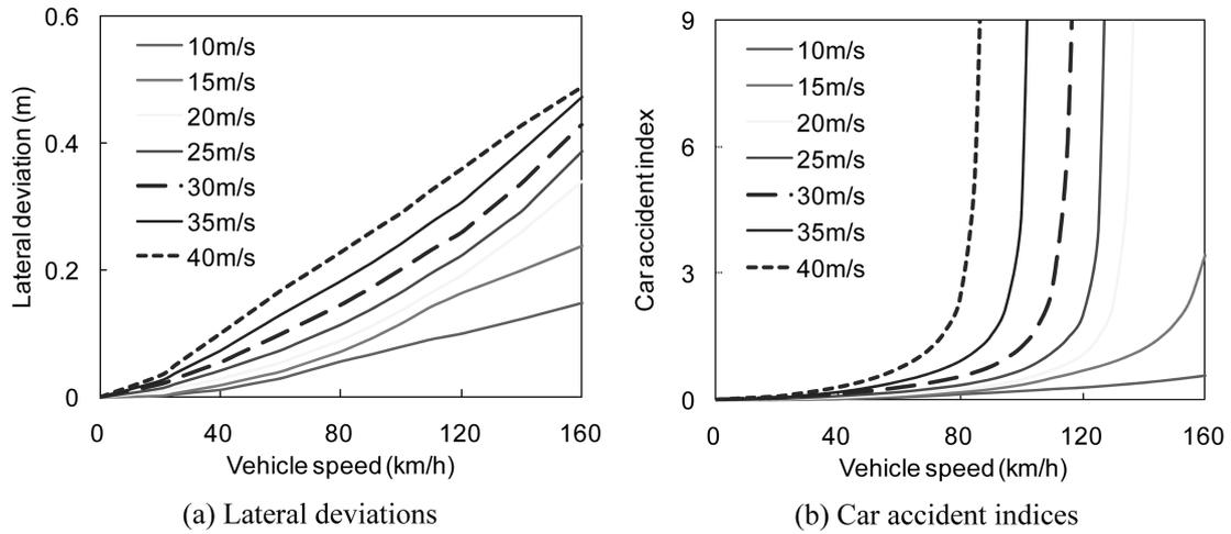
Fig. 8 Lateral deviations and their corresponding car accident indices of a truck according to wind speeds (dry condition)
