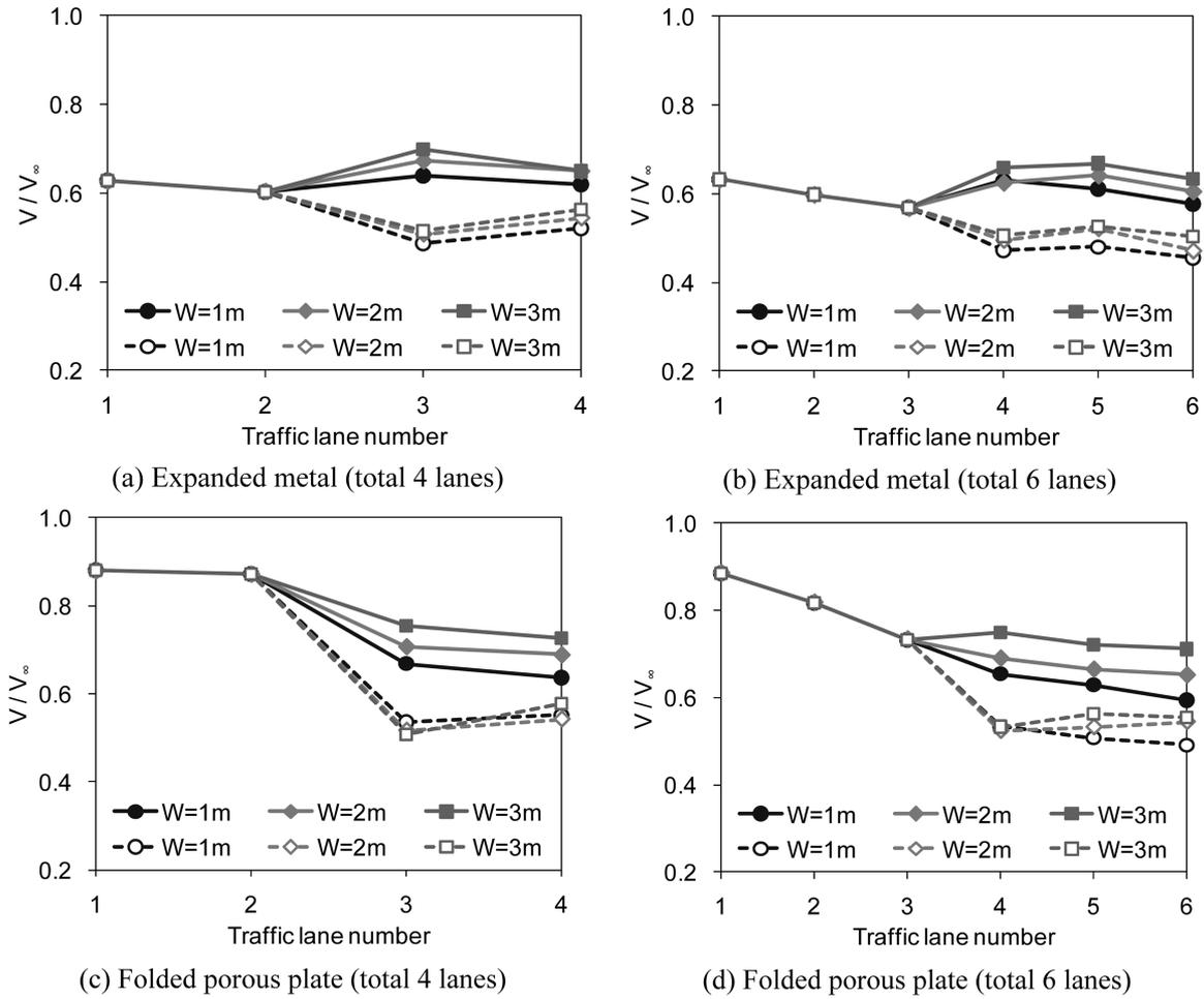
Fig. 16 Normalized wind velocities at 0.4 m above road at center of traffic lanes numbered from windward; solid line: C1, dotted line: C2
