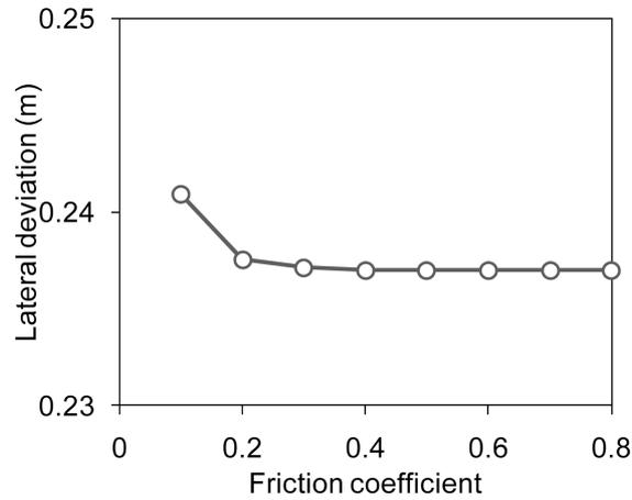
Fig. 6 Lateral deviations of a sedan under various friction coefficients of road surface
