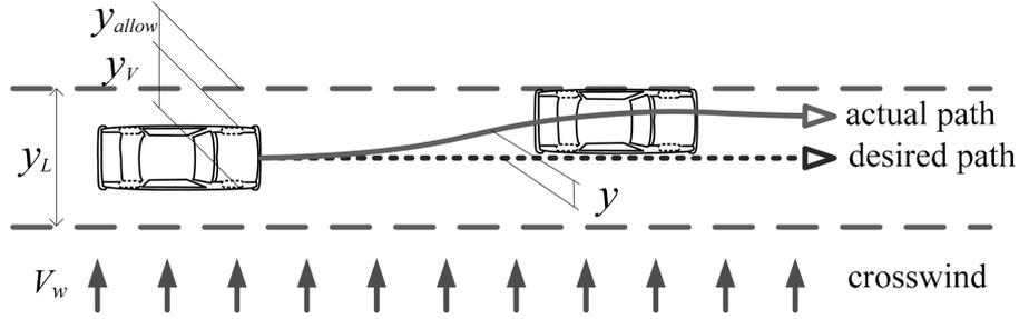
Fig. 3 Vehicle path under crosswind
