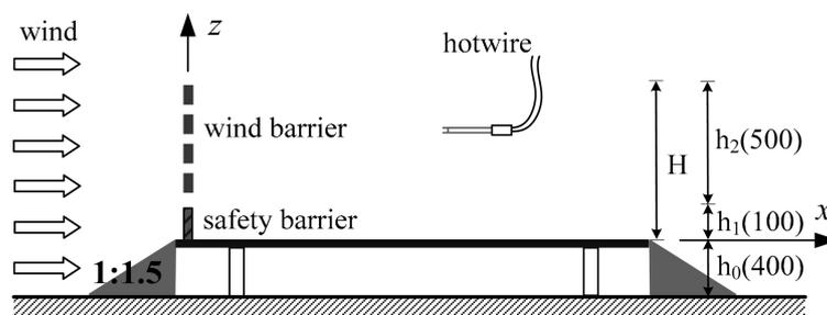
Fig. 10 Schematic diagram of wind barrier arrangements at elevated bridge and embankment
