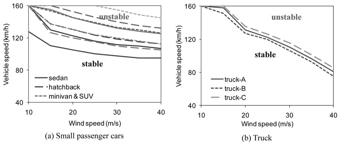
Fig. 9 Safety limits for driving stability of road vehicles
