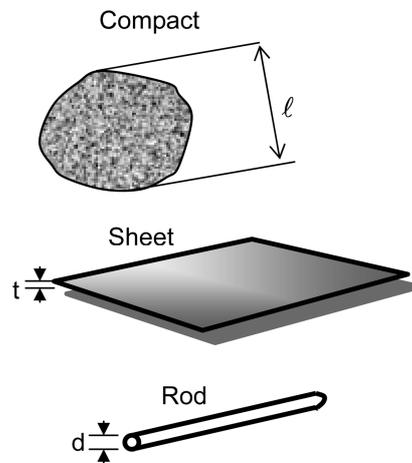
Fig. 2 Three generic debris types (Wills, *et al.* 2002)
