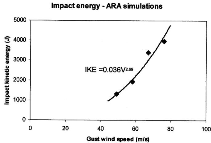
Fig. 5 Total impact kinetic energy as a function of maximum gust speed in a hurricane, from all windborne debris impacts in a representative U.S. subdivision (re-plotted from the results of Twisdale, *et al.* 1996)
