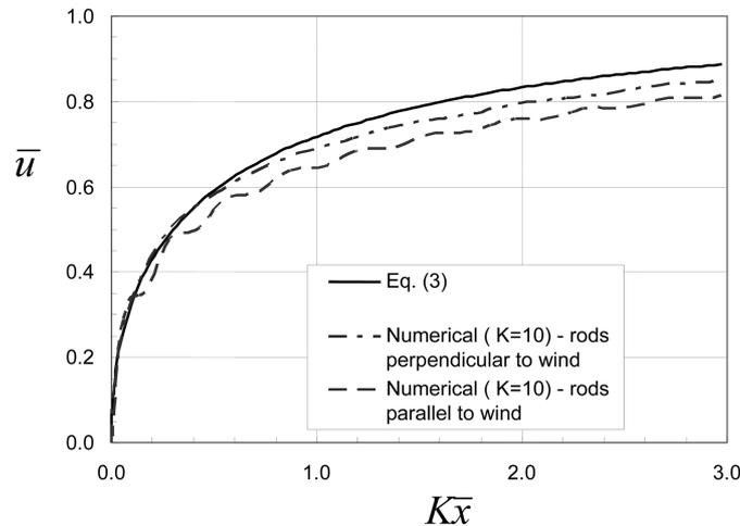
Fig. 3 Non dimensional horizontal missile velocity versus non dimensional distance traveled for rod-type objects (from Lin, *et al.* 2007)
