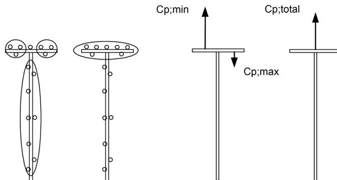
Fig. 6 Combined time series and definition of Cp-values for T-tops
