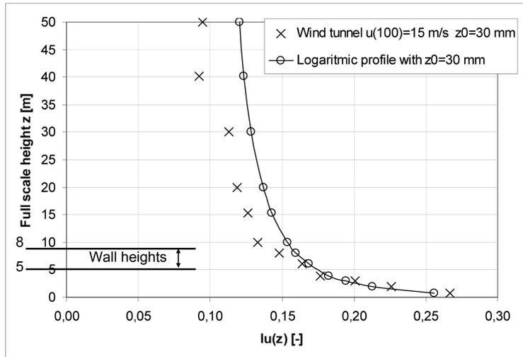
Fig. 2 Turbulence intensity from the wind tunnel
