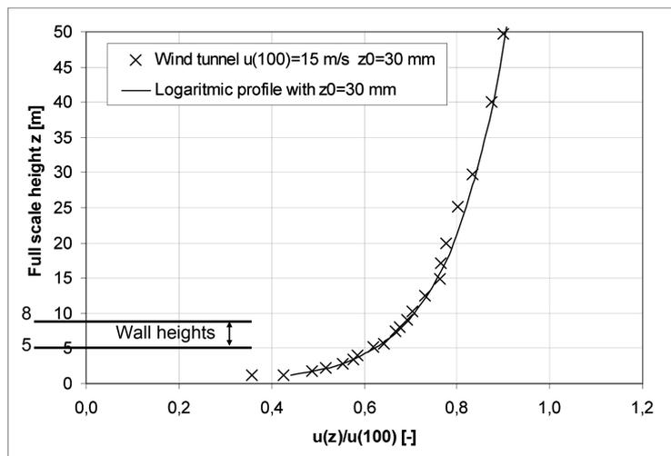
Fig. 1 Mean wind velocity from the wind tunnel
