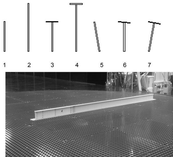
Fig. 3 Free-standing wall configurations (left); model in the wind tunnel (right)
