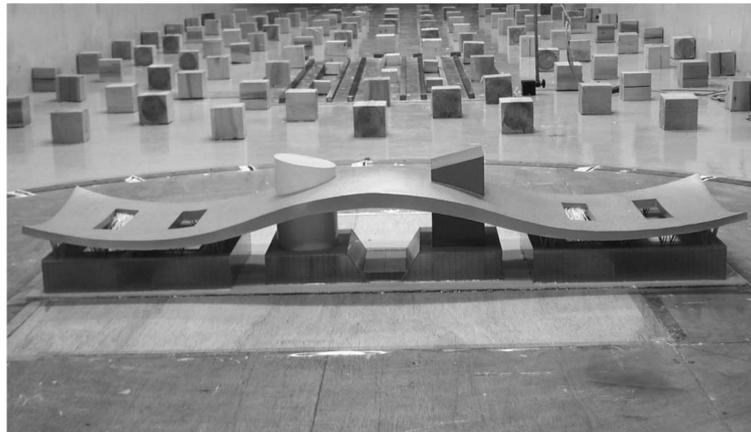
Fig. 1 Model of the SZCC in the wind tunnel test
