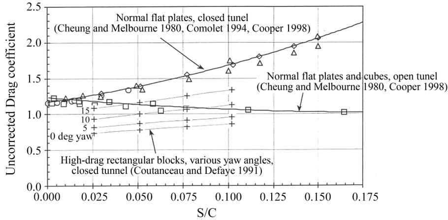
Fig. 5 Bluff-body blockage effects on drag in closed and open test sections (Cooper 1998)
