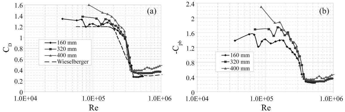
Fig. 3 Uncorrected drag coefficient (a) and uncorrected base pressure coefficient (b) evolutions
