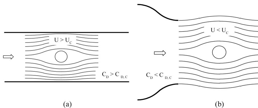
Fig. 4 Blockage effect in open (a) and closed (b) test section wind tunnels
