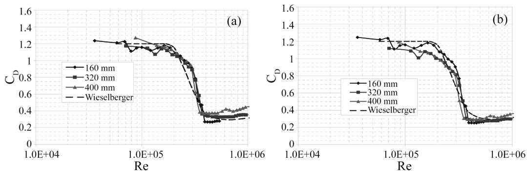
Fig. 7 Drag coefficient corrected by Maskell with  $\varepsilon = 0.96$  (a) and by Modi & El-Sherbiny (b)
