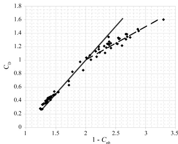
Fig. 8 Drag coefficient versus  $(1 - C_{pb})$  for circular cylinders
