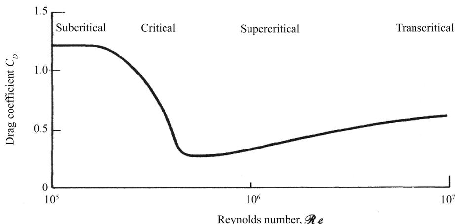
Fig. 1 Evolution of drag coefficient for circular cylinder from Simiu and Scanlan (1996)
