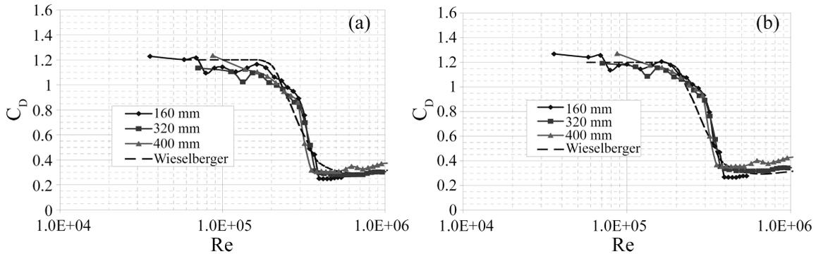
Fig. 6 Drag coefficient corrected by Glauert with  $G=0.6$  (a) and by Allen and Vincenti (b)
