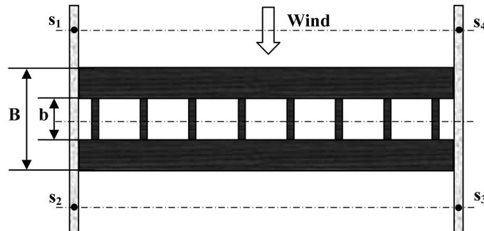
Fig. 4 Top view of model-rig system and the layout of laser sensors ( $s_1$ ,  $s_2$ ,  $s_3$  and  $s_4$ )
