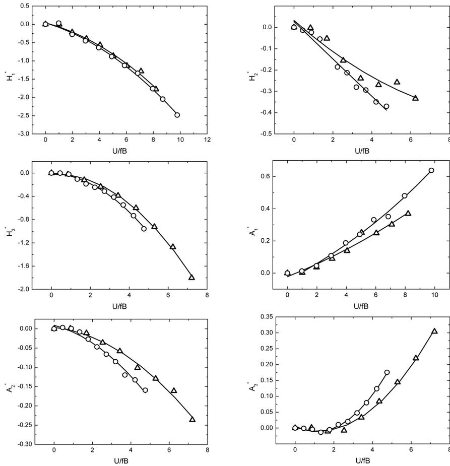
Fig. 6 Flutter derivatives of model with 16% gap-width
