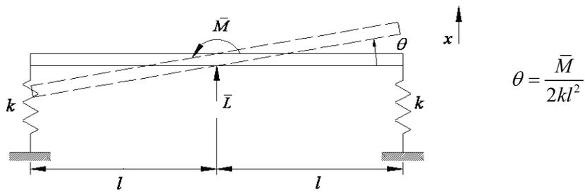
$\bar{M}$ : mean of pitching moment  $\bar{L}$ : mean of lift force  $\theta$ : additional angle of wind incidence
