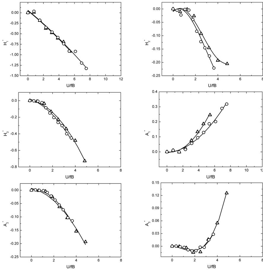
Fig. 7 Flutter derivatives of model with 35% gap-width
