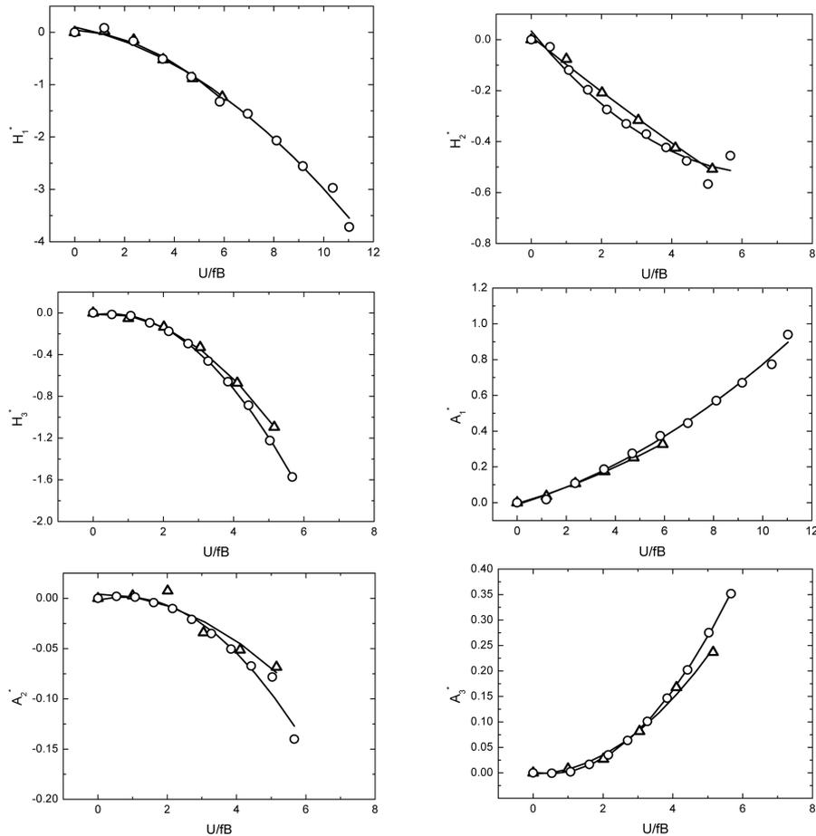
Fig. 5 Flutter derivatives of model with a zero gap-width
