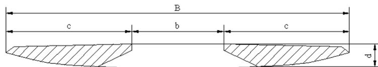
Fig. 3 Cross section shape of the bridge sectional models
