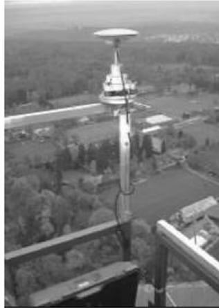
Fig. 3 The Stuttgart TV Tower with GPS-Antenna (Rover Station) mounted on the hand-rail of the balcony, 5 meters above viewing platform
