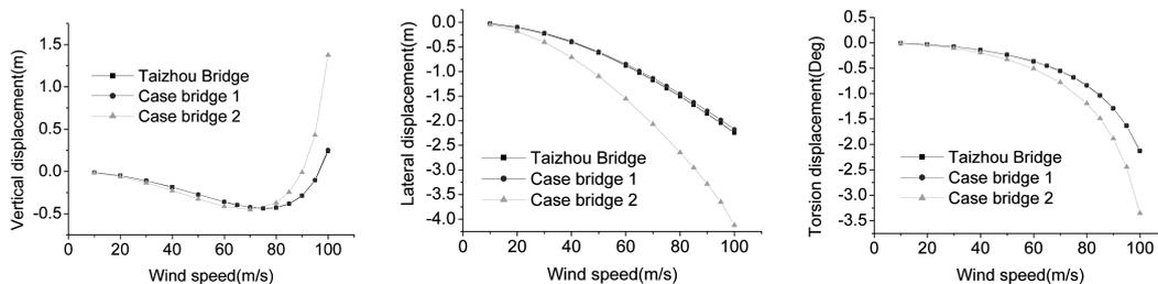
Fig. 2 Evolutions of the bridge deck's displacements at midpoint of main span with wind speed
