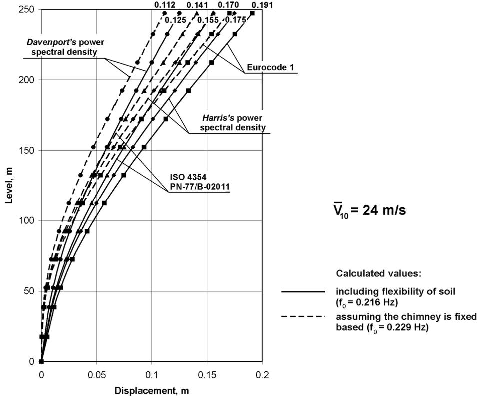
Fig. 5 Comparison of the along-wind displacements of the chimney with and without flexibility of soil for  $\bar{V}_{10} = 24$  m/s
