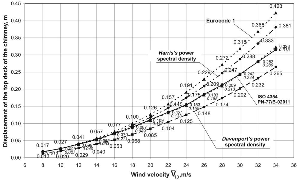
Fig. 2 Comparison of the top deck chimney along-wind displacements for different values of  $\bar{V}_{10}$
