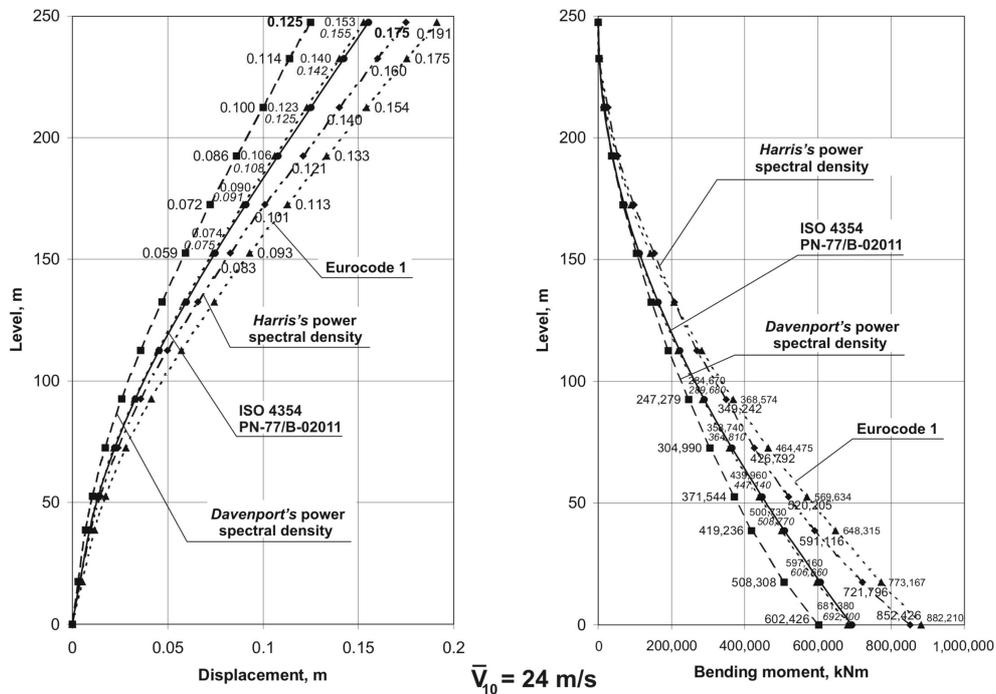
Fig. 1 Comparison of the along-wind displacements and bending moments of the chimney for  $\bar{V}_{10} = 24 \text{ m/s}$
