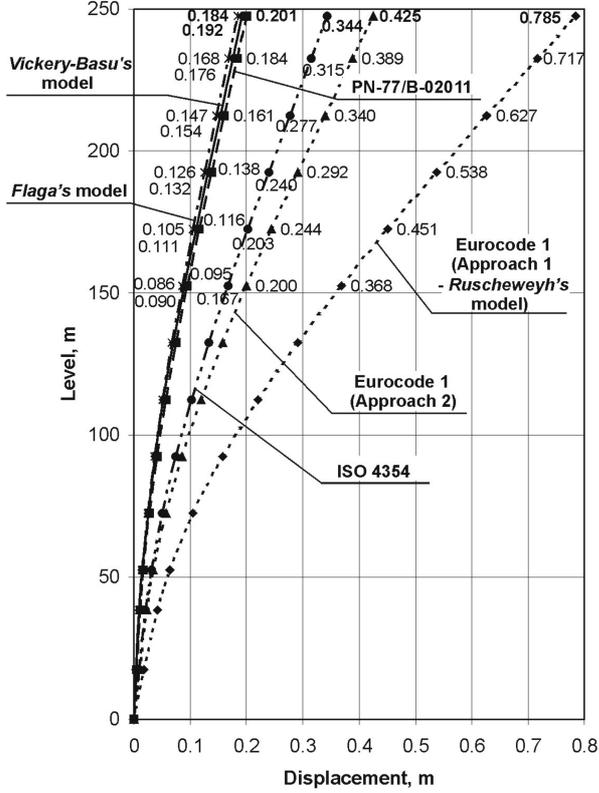
Fig. 3 Comparison of the cross-wind chimney displacements for  $V_{cr} = 25.9$  m/s ( $St = 0.2$ )
