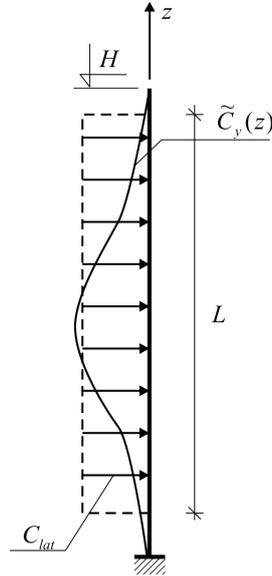
Fig. 7 Ruscheweyh's model for cross-wind excitation of a slender structure
