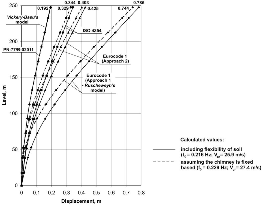
Fig. 6 Comparison of the cross-wind displacements of the chimney with and without flexibility of soil for  $V_{cr} = 25.9$  m/s ( $St = 0.2$ )
