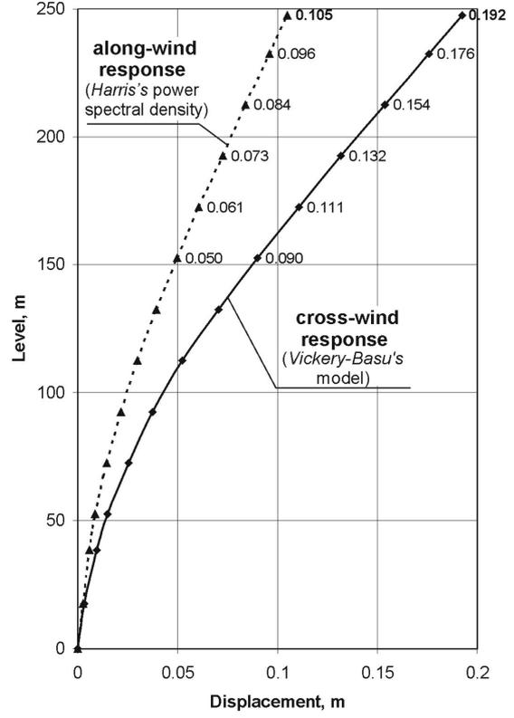
Fig. 4 Comparison of the along and cross-wind chimney displacements for  $V_{cr} = 25.9$  m/s ( $\bar{V}_{10} = 19$  m/s,  $St = 0.2$ )
