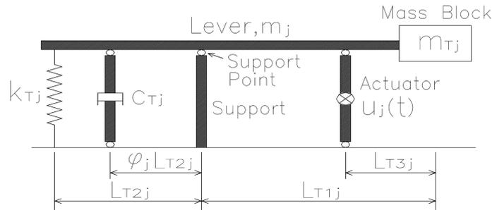
Fig. 2 Schematic diagram of the  $j$ th LT-ATMD in the LT-AMTMD with the damping set at the position between the spring and the support
