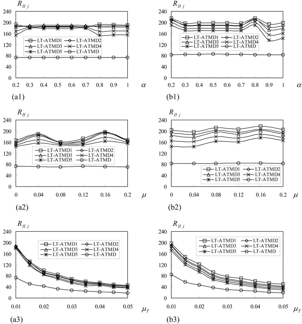
Fig. 6 Variation of the  $R_{IIj}$  value of the LT-AMTMD (including the LT-ATMD) with respect to the  $\alpha$  value with  $n=5$  and  $\mu_T=0.01$  and  $\mu=0.03$  [(a1):  $r=-0.4$ ; (b1):  $r=-0.8$ ] and the  $\mu$  value with  $n=5$  and  $\mu_T=0.01$  and  $\alpha=0.3$  [(a2):  $r=-0.4$ ; (b2):  $r=-0.8$ ] and the  $\mu_T$  value with  $n=5$  and  $\alpha=0.3$  and  $\mu=0.03$  [(a3):  $r=-0.4$ ; (b3):  $r=-0.8$ ]
