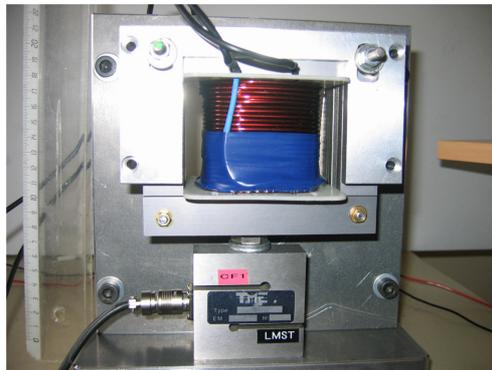
Fig. 3 Experimental arrangement for the actuator identification
