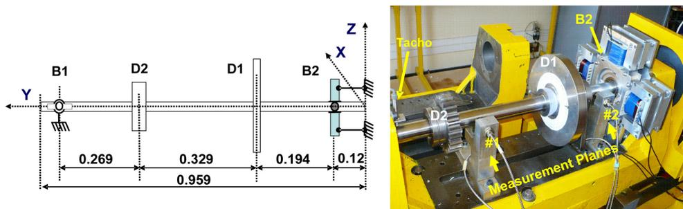
Fig. 1 Experimental test rig
