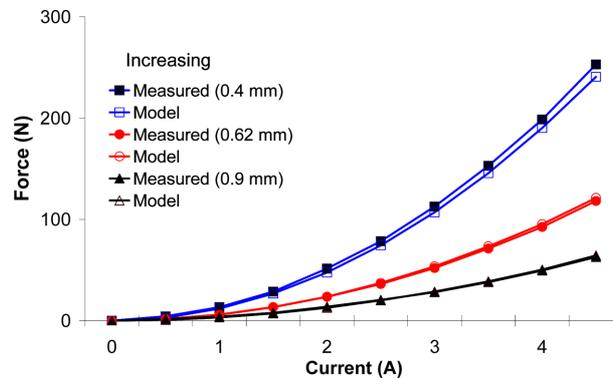
Fig. 5 Measured and calculated forces versus current for several air gaps
