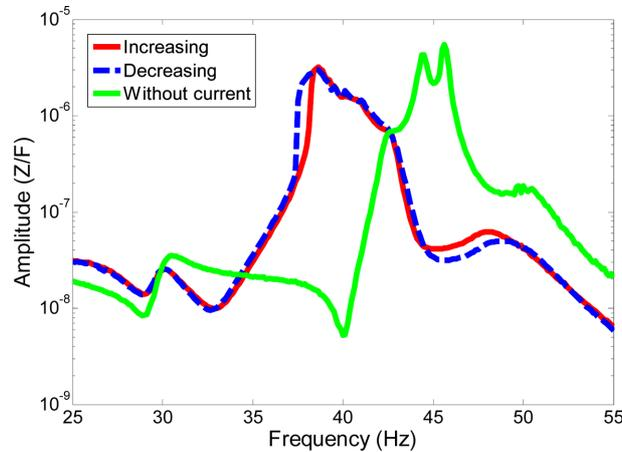
Fig. 6 Transfer function, C3, sinusoidal sweep, with and without current
