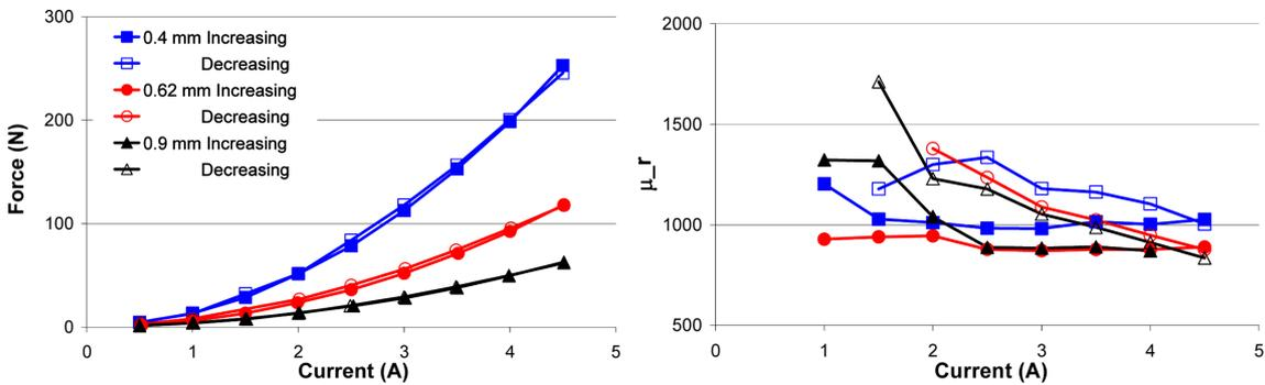
Fig. 4 Measured forces and relative permeability versus current for several air gaps
