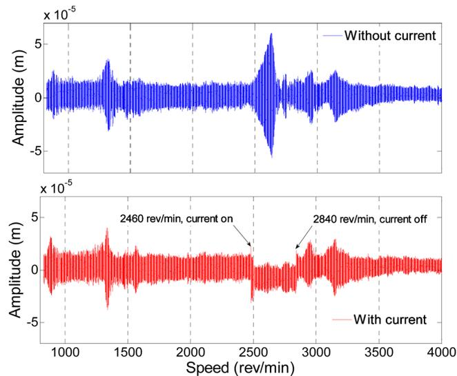
Fig. 8 Displacement amplitude, C2, run-up
