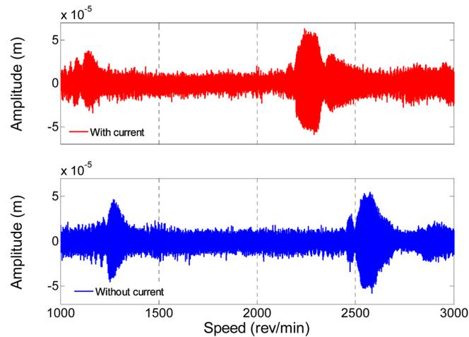
Fig. 7 Displacement amplitude, C2, 800 to 4000 rev/min in 30 sec
