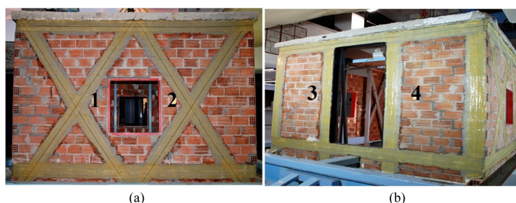
Fig. 7 A picture of the repaired masonry building with reinforced GFRP strips: (a) sides 1-2 and (b) sides 3-4
