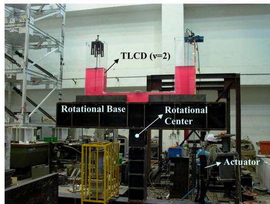
Fig. 5 Picture of a TLCD on the rotational base
