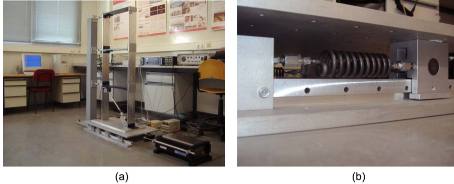
Fig. 1 (a) Plane frame physical model supported by a shaking table and (b) detail of the shaking table
