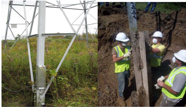
Fig. 6 NDE system during inspection of transmission line stub angle (left) and acutal excavation and inspection (right)
