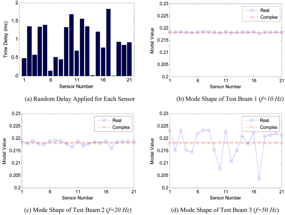
Fig. 11 Mode shape of three test beams for random time-delay
