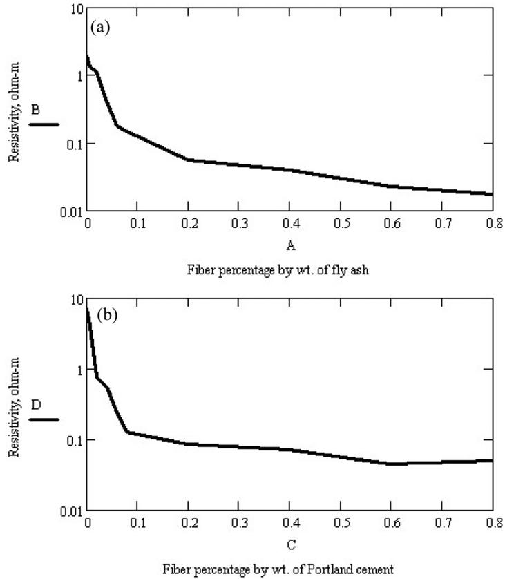
Fig. 7 Resistivity of the specimen vs. fiber percentage by weight of cementitious binder, (a) Geopolymer cement mortar and (b) Portland cement mortar
