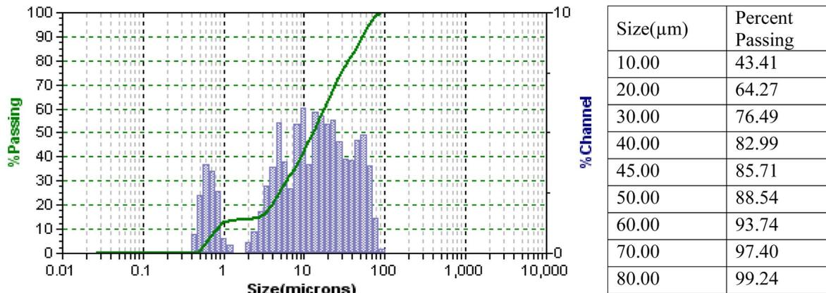
Fig. 3 Particle size distribution of fly ash stockpile
