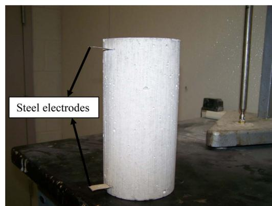
Fig. 6 Concrete cylinder specimen with embedded steel electrodes
