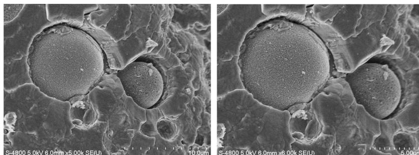
Fig. 1 SEM images of geopolymer showing unreacted fly ash particles surrounded aluminosilicate binder
