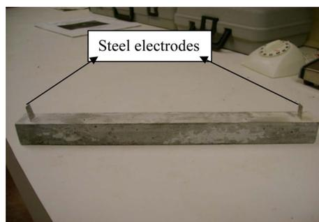
Fig. 2 A rectangular bar specimen with embedded steel electrodes
