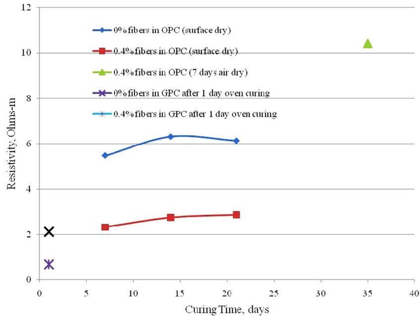
Fig. 8 Resistivity of concrete specimens vs. curing time
