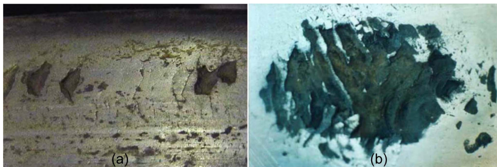
Fig. 4 Wheel tread (a) spalling and (b) shelling (Zakharov and Goryacheva 2005)
