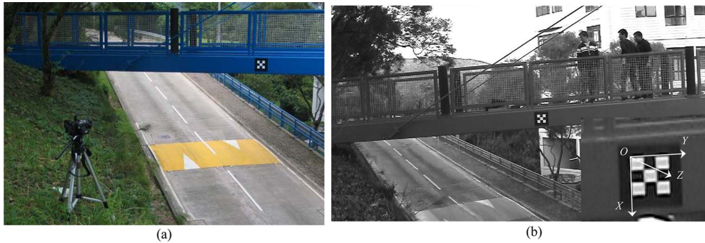
Fig. 10 (a) Test setup and (b) first image recorded by the camera and an enlarged image showing the planar target with a corner-fixed world coordinate system
