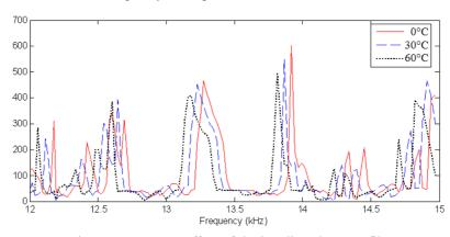
Fig. 8 Temperature effect of the baseline phase profile
