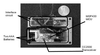
Fig. 6 Prototype of ASN-2 developed using a TI MSP430 evaluation board
