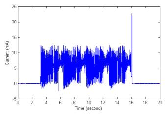
Fig. 12 Measured current profile of ASN-2 during an SHM operation
