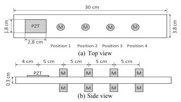
Fig. 9 Test structure and positions of magnets
