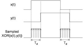
Fig. 3 Phase difference measured by sampling the output of the XOR operation
