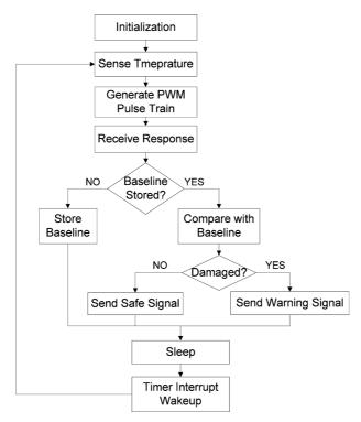
Fig. 7 system operation flow of ASN-2
