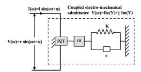
Fig. 1 Model of an impedance-based SHM
