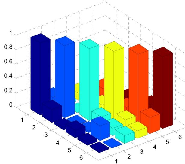
Fig. 4 MAC matrix between the first 6 mode shapes in the first optimal 10 DOFs
