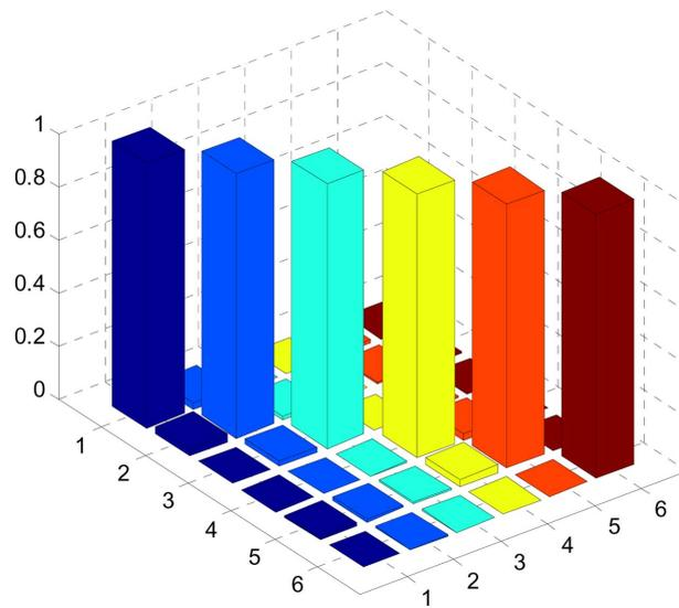
Fig. 5 MAC matrix between the first 6 mode shapes in the first optimal 15 DOFs
