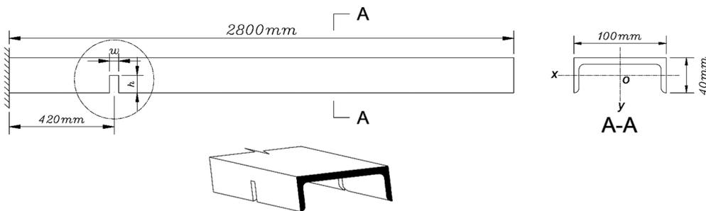
Fig. 8 Dimensions and plans of experimental cantilever beam
