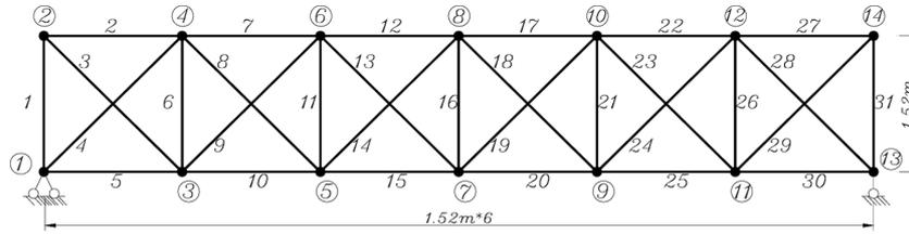
Fig. 2 Finite element model of a simply supported, 6-bay planar truss
