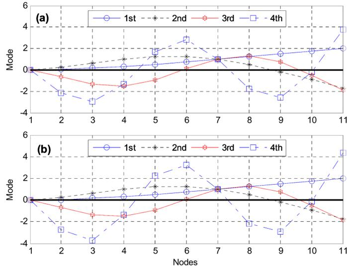
Fig. 11 The first 4 mode shapes of the undamaged (a) and damaged (b) cantilever beam
