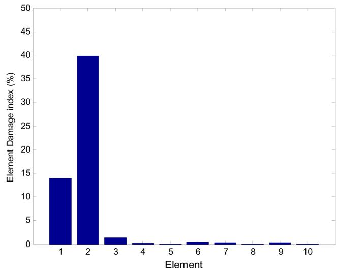
Fig. 12 Element damage index for the FE model
