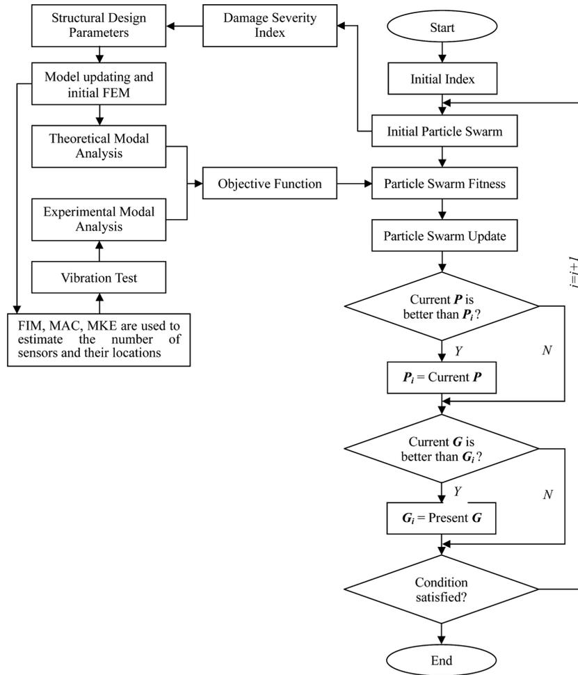
Fig. 1 Damage detection algorithm flowchart
