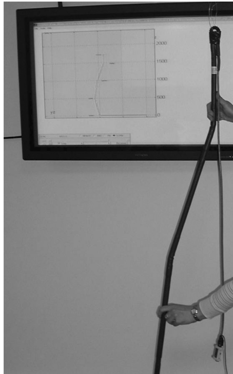
Fig. 1 Photograph of the wireless ShapeAccelArray and corresponding visualization of sensor positions
