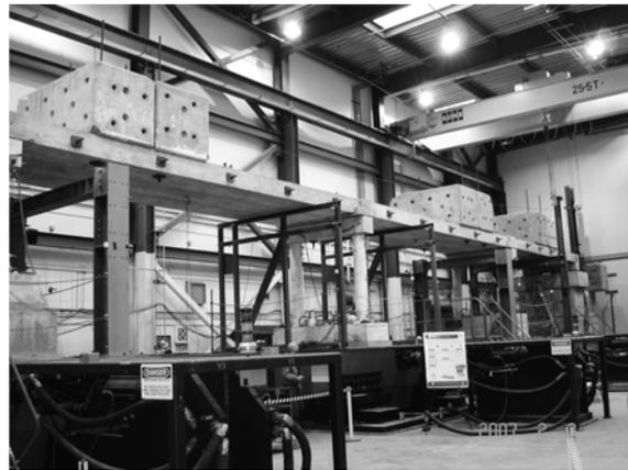
Fig. 2 Bridge on the shaking tables
