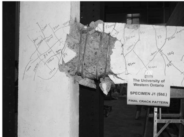
Fig. 5 Final crack pattern for the standard steel-reinforced specimen *J1*
