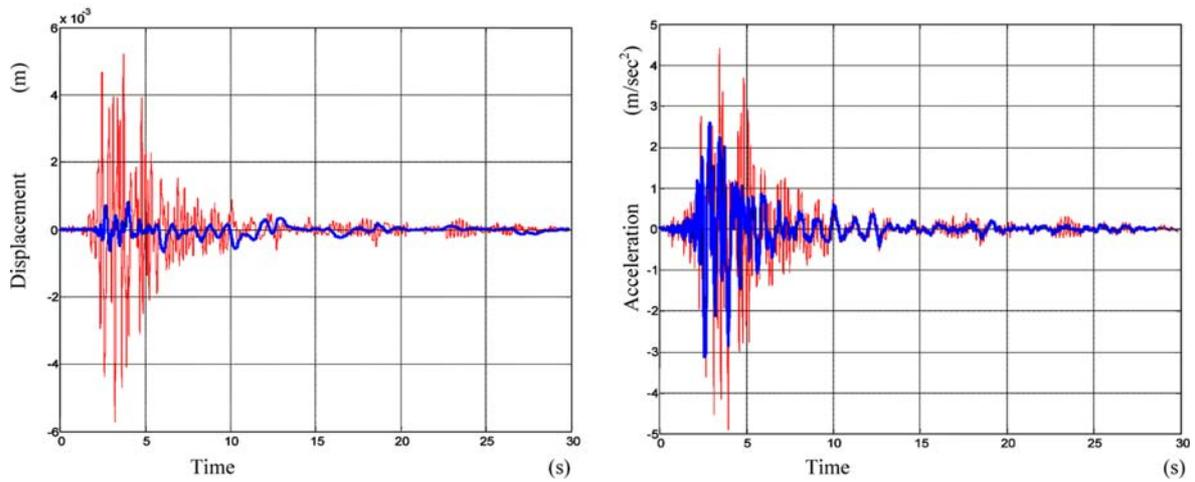
Fig. 8 Displacement and acceleration of controlled (bold line) and uncontrolled (thin line) system for single degree-of-freedom structure subjected to Kalamata (1986) earthquake
