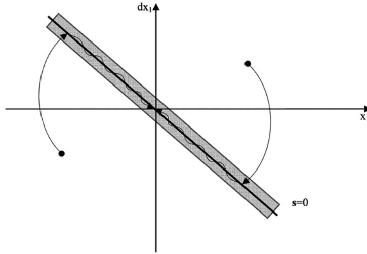
Fig. 5 The movement of the system's trajectory towards to sliding surface and next to the equilibrium point
