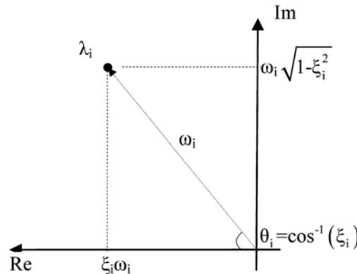
Fig. 2 Representation of the poles of the structure in the complex plane
