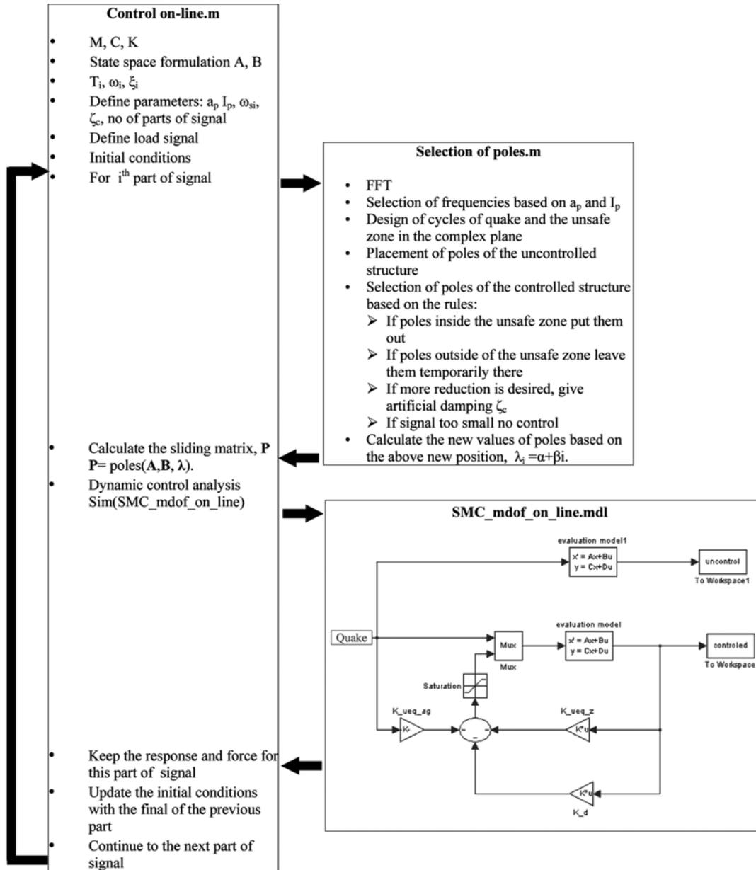
Fig. 6 The control strategy based on sliding mode control algorithm suitable for buildings subjected to earthquake actions
