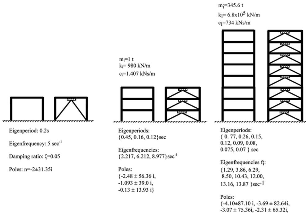
Fig. 7 The simulation models and their dynamic characteristics
