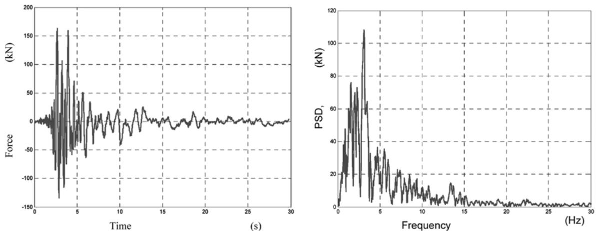
Fig. 9 The demanded force and the Power Spectral Density, PSD, of force for single degree-of-freedom structure subjected to Kalamata (1986) earthquake
