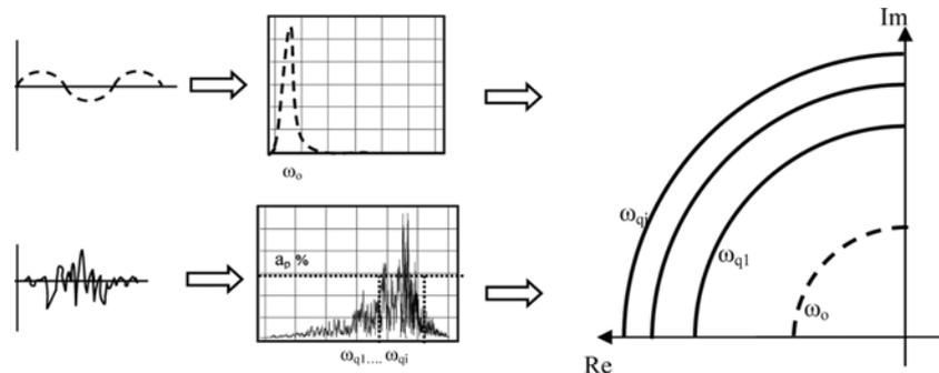
Fig. 3 Representation of frequencies of two types of loading, sinusoidal and earthquake, by cycles in the complex plane
