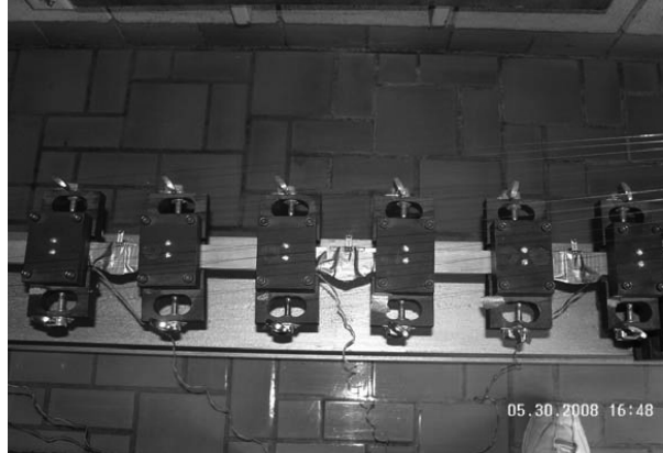
Fig. 12 Piezo-elements on model bridge as vibration sensors
