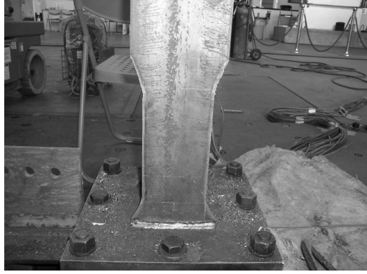
Fig. 2 Photograph of the cut flanges of the column
