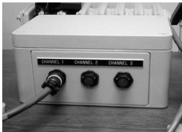
Fig. 5 The three channels conjunction box
