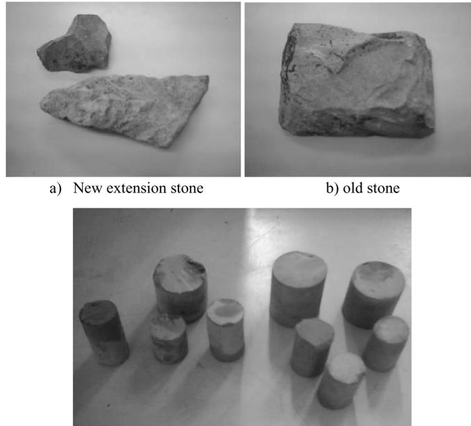
Fig. 3 Two stone samples taken from the old and new part of the minaret
