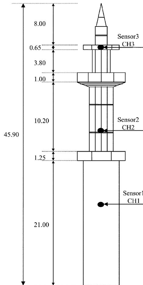
Fig. 7 Location of the three sensors
