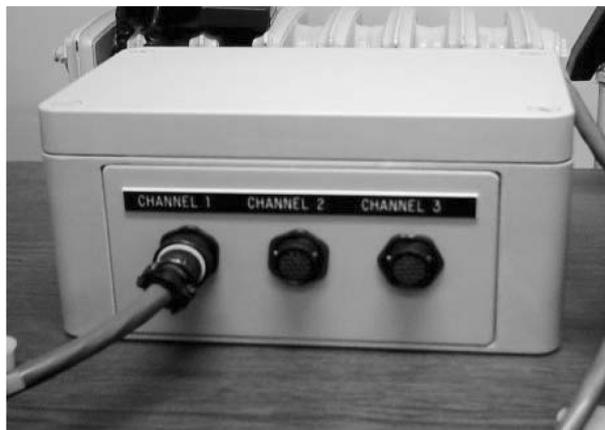
Fig. 5 The three channels conjunction box
