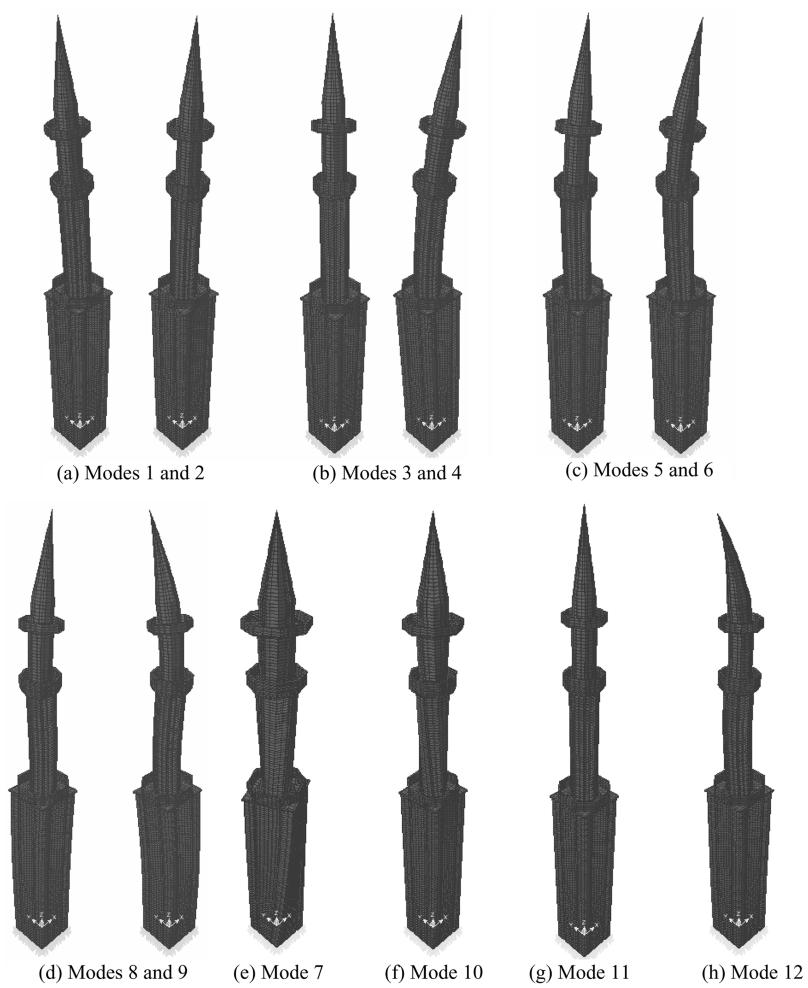
Fig. 12 Analytical first 12 mode shapes
