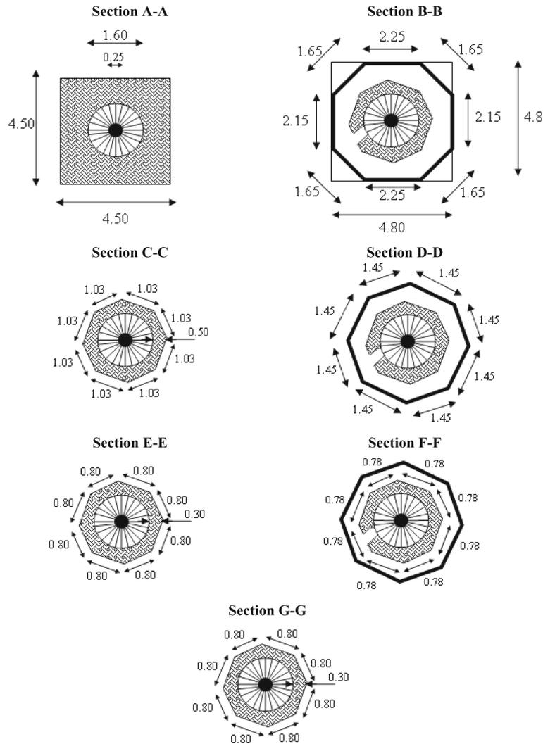
Fig. 2 Different section of the minaret
