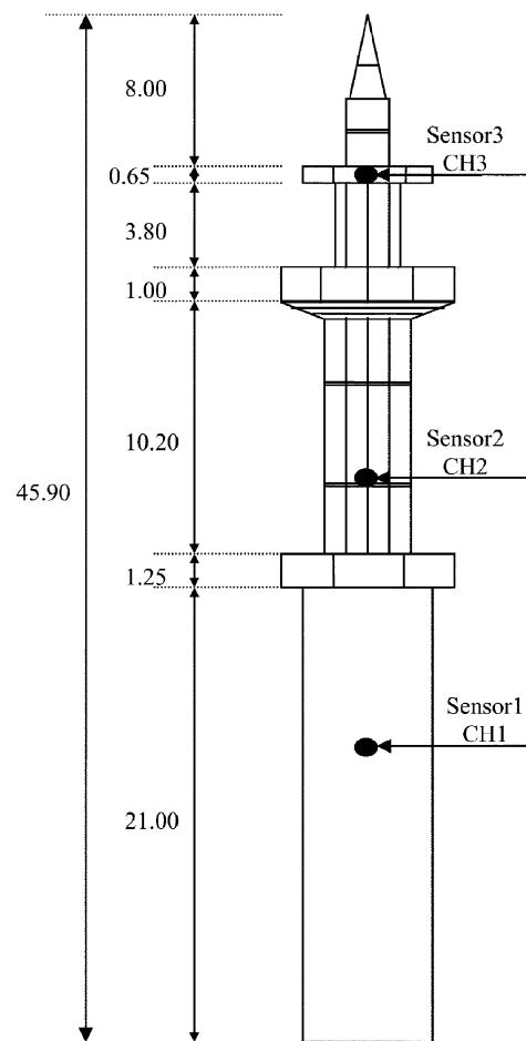
Fig. 7 Location of the three sensors
