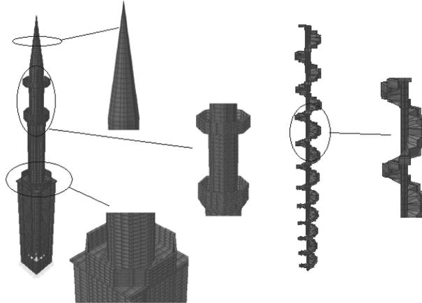
Fig. 11 Details of three dimensional finite element model of the minaret
