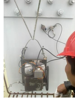
Fig. 14 Vibration exciter for forced vibration tests of the damping ratios of hanger-TMD System
