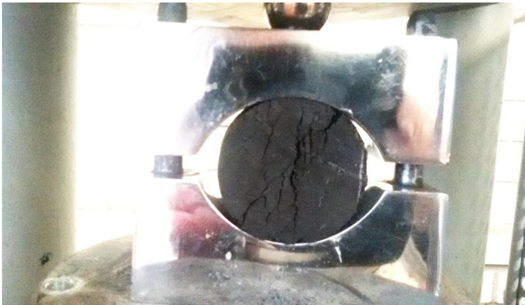
Fig. 3 Failure pattern in Brazilian test
