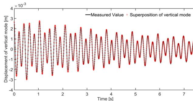
Fig. 18 Time history data of superposed vertical mode using the ILS method and FIVP
