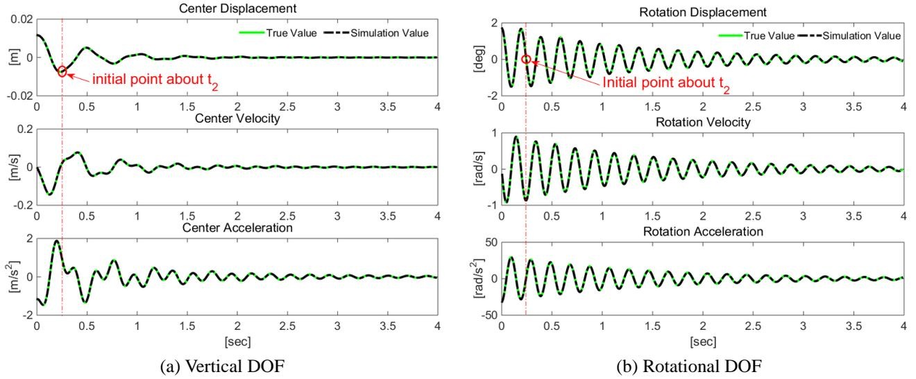
Fig. 1 Comparison between true and simulated values for 2DOF in time domain using the ILS method and the original initial condition (system 1)
