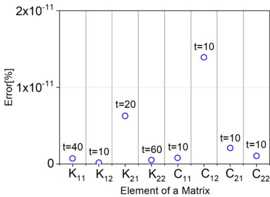
Fig. 3 The accuracy of the free initial value problem compared with the original initial value problem (Each number on the circle-symbol indicates the time [s] of occurrence)
