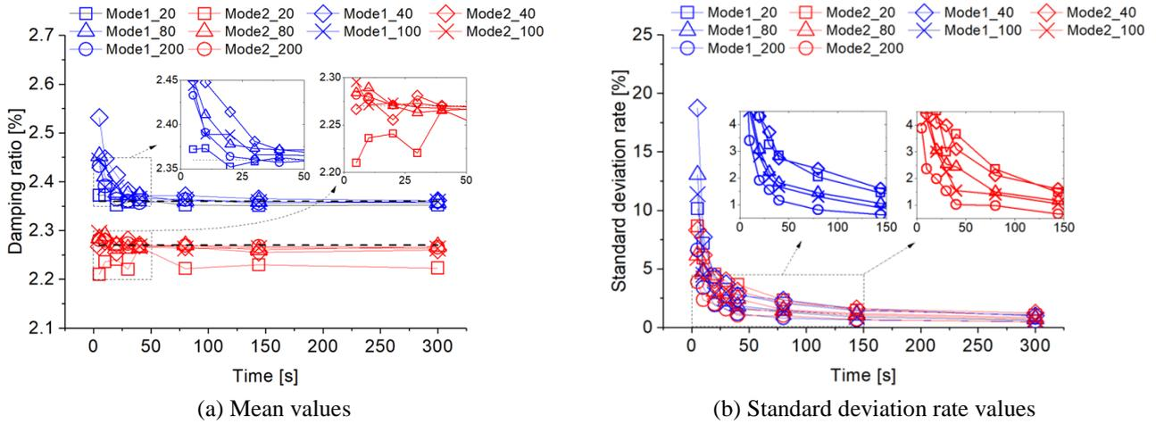
Fig. 7 Mean and standard deviation rate of modal damping ratio for each case of SM1 (mode 1 represented by blue lines, mode 2 by red lines; dashed lines present theoretical values)
