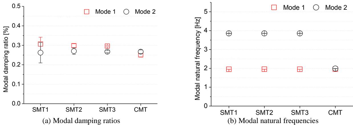
Fig. 14 Mean and standard deviations of damping ratio and frequency under 40 s and 120 Hz for all models in section model tests
