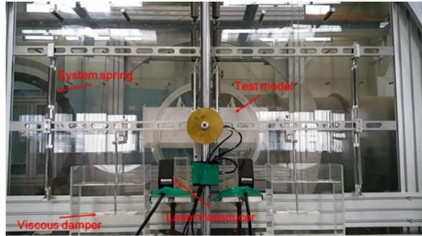
Fig. 9 Test set-up for free and ambient vibrations for vertical and torsional mode in Korea university
