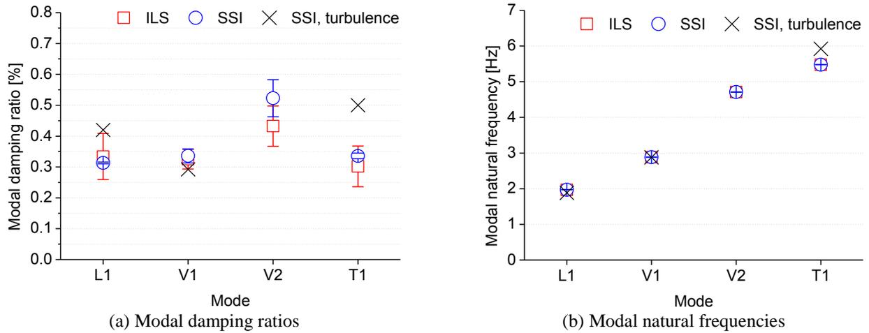
Fig. 16 Mean and standard deviation of modal damping ratio and frequency under 60 s and 200 Hz for all modes, using the ILS and SSI method in full bridge 3D model tests
