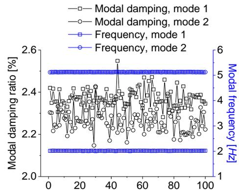
Fig. 6 Numerical simulation of case 3e with modal damping ratio and natural frequency for two modes
