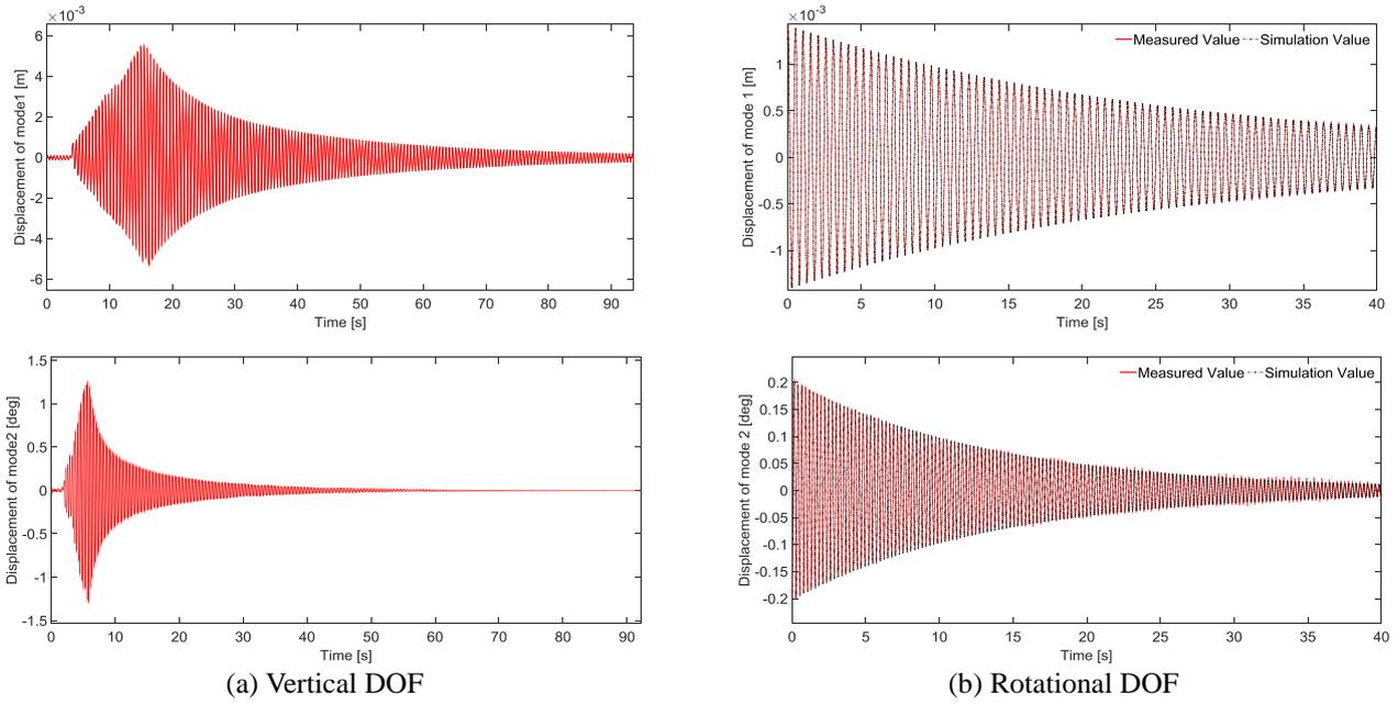
Fig. 12 Time history displacement data using the ILS method under 40 s and 120 Hz in SMT 3 for all modes (simulation values were compared with measured values)
