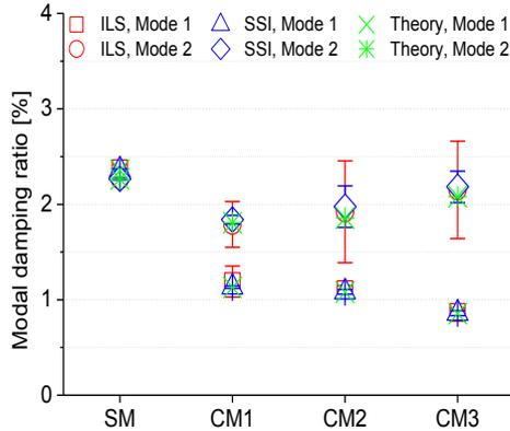
Fig. 8 Mean and standard deviation of modal damping ratio of case 3e with two modes for all numerical models (the ILS method in red, the SSI method in blue, and theoretical values in green)
