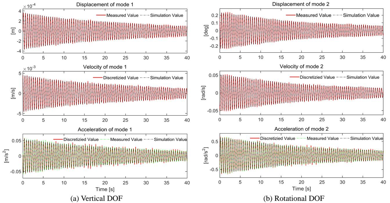
Fig. 13 Time history displacement data using ILS method under 40 s and 120 Hz in CMT for all modes (displacement at the top, velocity in the middle, acceleration at the bottom; simulation values were compared with measured values)
