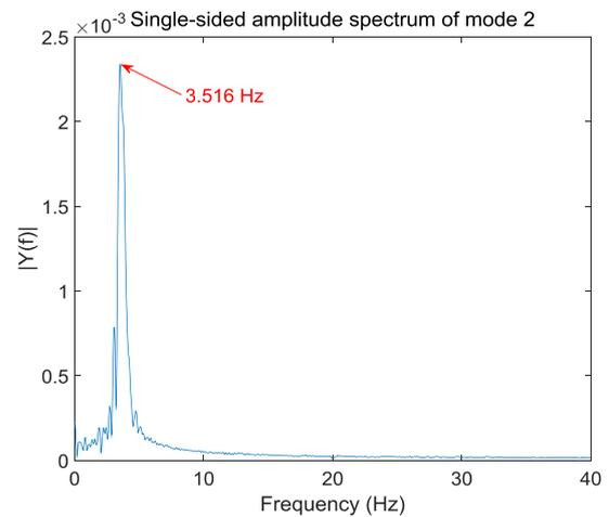
Fig. 11 FFT diagram of subjected forces for each DOF (mode 1 in left, mode 2 in right)
