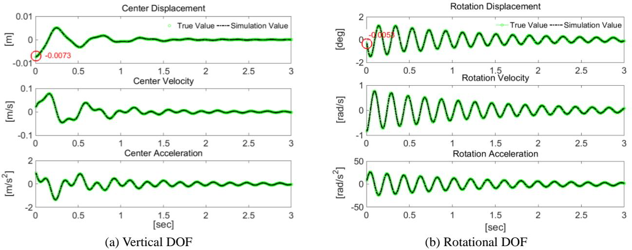
Fig. 2 Comparison between true and simulated values for 2DOF in time domain using the ILS method and the free initial condition (system 2)
