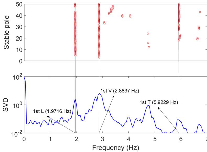
Fig. 17 SVD and stabilization diagram obtained with the SSI method in full bridge 3D model tests
