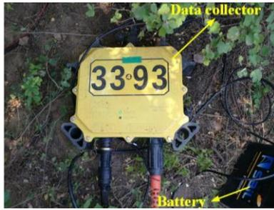
Fig. 7 Data collector and battery
