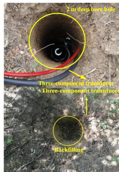
Fig. 6 Installation of transducers on surface
