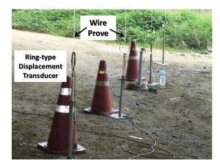
Fig. 2 Field application of ring gauges using tensioned wire as an extended probe
